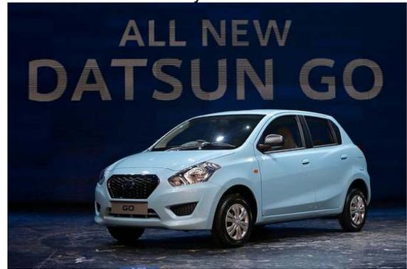
The car will cost less than 400,000 rupees (\$6,680).. The GO is a five-door hatchback with a manual transmission, and is powered by a 1.2-liter engine. The car is less than four meters long, which means it qualifies for a lower 12% excise tax in India.
