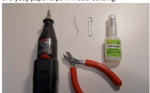
Sometimes there are glue joints that need some extra support for joint strenght or positioning. I often use paper clips for this. You only need a paper clip (more accuratly a portion of one), a drill and your adhesive of choice.
