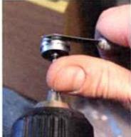
I had to sand a little away the first time to get the thickness right to fit the Slot.IT wheel depth.
