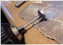
Once the fit is just right, turn the wheel on the razor saw to cut off the hub, trim and drill a hole right in the center to accommodate the hub.
