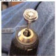
holding the razor saw steady, just in front of the center ridge, turn the wheel until it cuts clean through.
