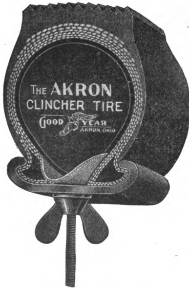
Fig. 6—Proper Position of Tire on Rim.
