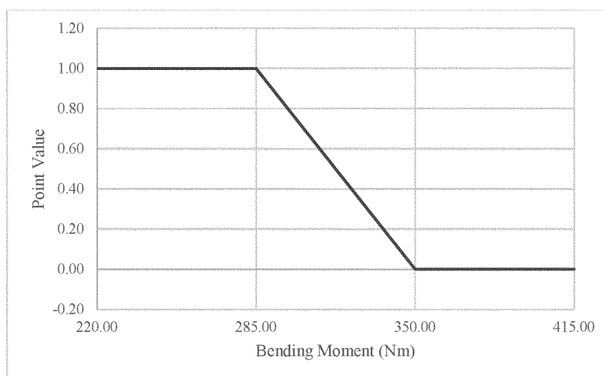
Figure 13: Upper Legform Bending Moment Scoring
