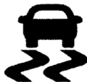
Figure 3: ESC Malfunction Telltale Symbol in FMVSS No. 101
