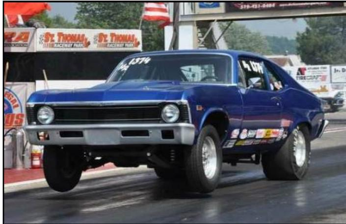
Racing since the late 1970's, Harry acquired this Nova in 1985. It has a 468 for power and is capable of runs in the 10.30 range.
