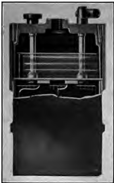
FIG. 173.—Special storage battery for airplane service.
