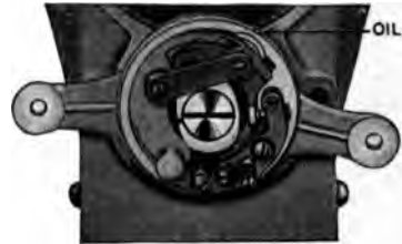
FIG. 285.—Point for oiling breaker arm on Aero magneto.
