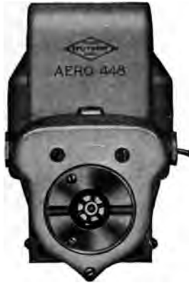
FIG. 288.—Rear view of Aero magneto showing impulse starter.
