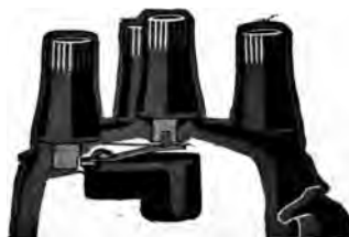
FIG. 104.—Construction of Atwater-Kent distributor head, type CC.
