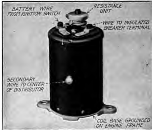
FIG. 119.—Remy induction coil—two primary terminal type.
