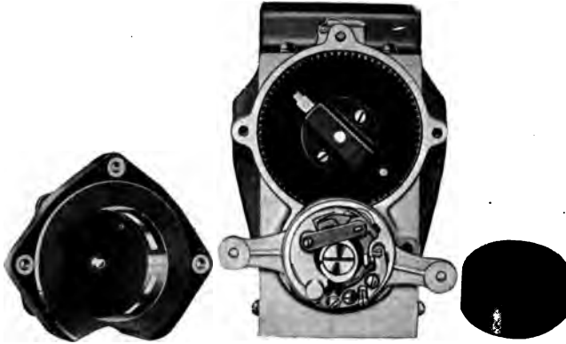
Fig. 281.—Aero magneto with distributor block and interrupter cover removed.
