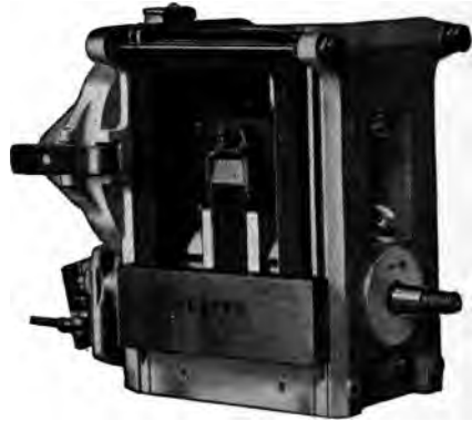
FIG. 341.—Keeper on magnet in Aero magneto.
