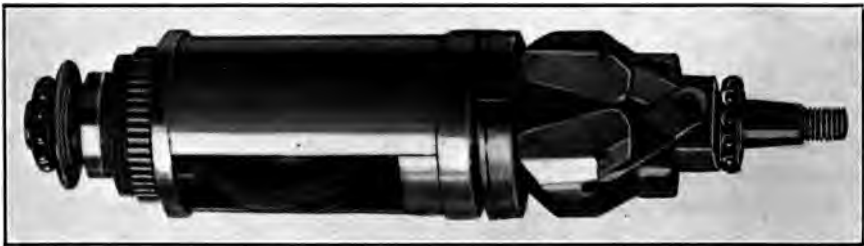
FIG. 235.—Eisemann magneto armature showing automatic spark advance mechanism.
