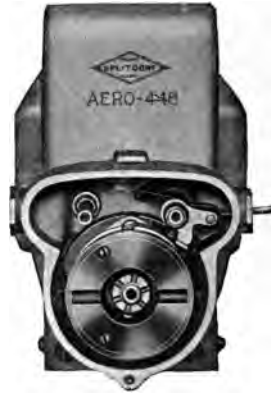
FIG. 289.—Rear view of Aero magneto with impulse starter cover removed.
