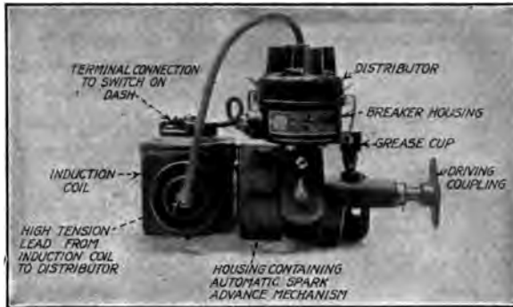
FIG. 127.—North East ignition unit.
