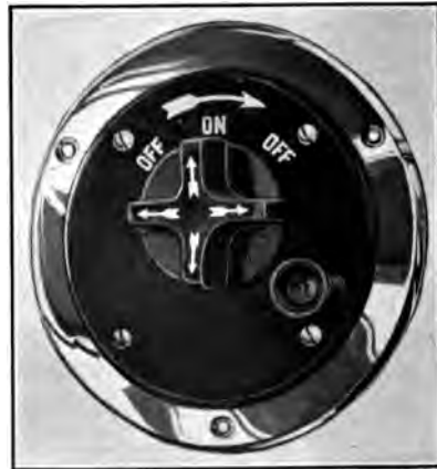
FIG. 97.—Atwater-Kent polarity reversing ignition switch.
