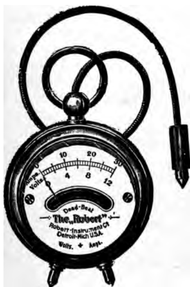
FIG. 28.—Typical pocket volt-ammeter for testing dry cells.
