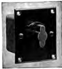
FIG. 136.—Front view, Westinghouse ignition switch.
