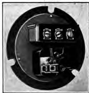
FIG. 115.—Rear view of Connecticut combination ignition and lighting switch, type KVD.
