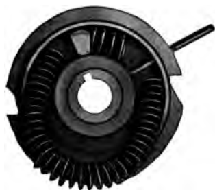
FIG. 291.—Springs used in Aero impulse starter.
