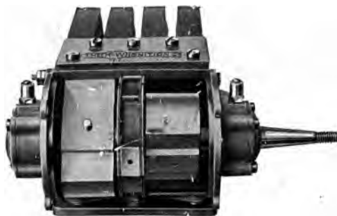
FIG. 255.—Interior view of K-W magneto showing rotor and coil.
