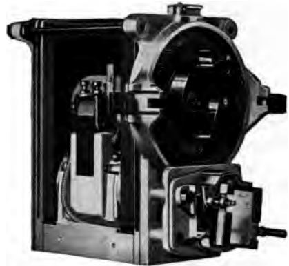
FIG. 301.—Interior view of Aero model 825 magneto.
