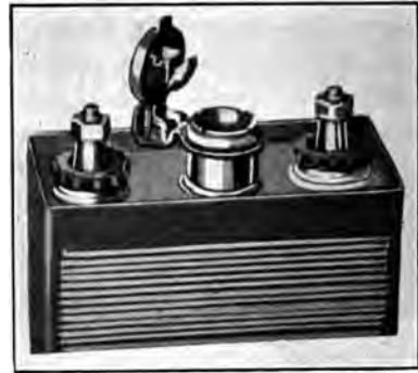
FIG. 36.—Top of Edison storage cell showing filling aperture open for adding water.
