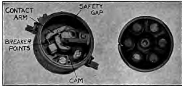
FIG. 121.—Remy breaker and distributor.
