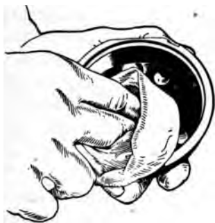
FIG. 92.—Method of cleaning distributor head.
