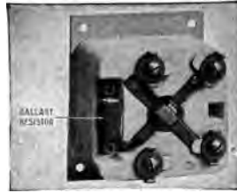
FIG. 137.—Rear view, Westinghouse ignition switch with resistor ballast mounted in place.
