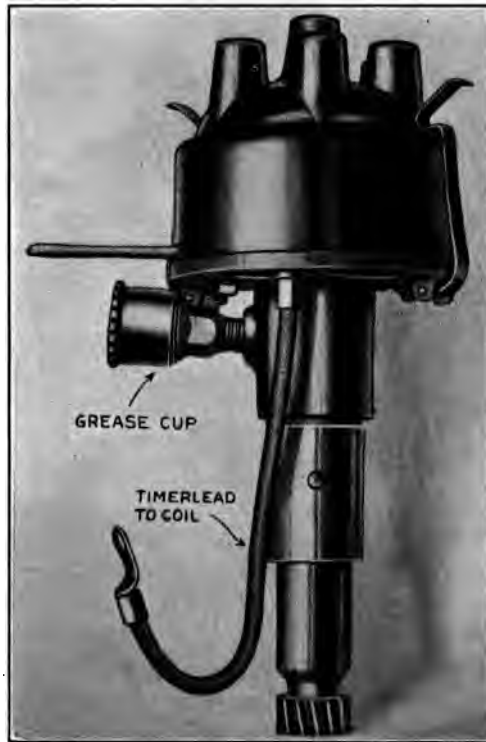
FIG. 149 e .—Complete Wagner timer distributor.
