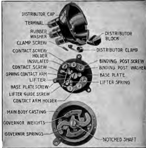
FIG. 95.—Construction of Atwater-Kent ignition unit, type K-2.
