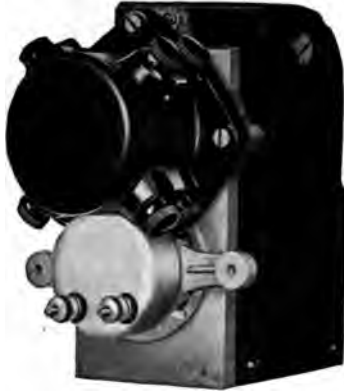
FIG. 294.—Aero magneto for eight-cylinder engines.
