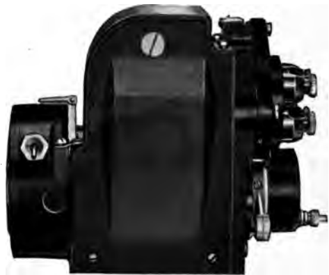
FIG. 287.—Aero Model 448 magneto fitted with impulse starter.
