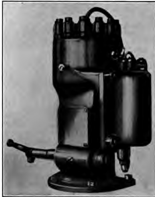
FIG. 149.—Philbrin distributor unit for twelve-cylinder engine, with coil mounted on base.
