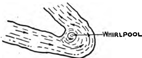
FIG. 23.—Water analogy of magnetic whirl around a conductor.
