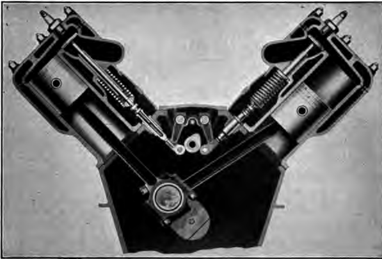
FIG. 152.—Sectional view of Cadillac eight-cylinder engine.
