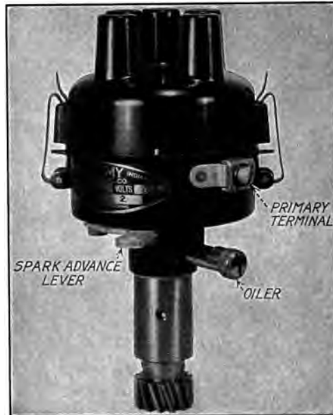
Fig. 125.—Remy-Liberty battery ignition unit for U. S. Military truck, Class B.
