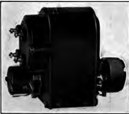
FIG. 244.—Kingston high-tension magneto, model O, showing impulse starter at right.
