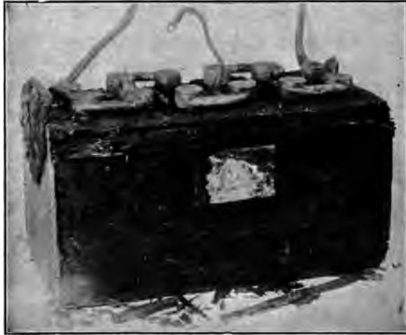
FIG. 63.—Effect of over-filling the battery cells.
