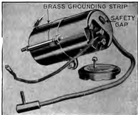
Fig. 109.—Connecticut coil showing spark gap and connections.
