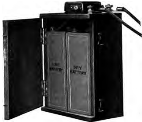
FIG. 305.—Buzzer test set for setting rotor edge distance.
