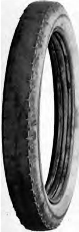
This is how a tire should wear out. The tread has been worn down evenly to the fabric just as you would wear out the sole of a shoe. The tire shown covered 11,800 miles. The credit for the performance should be equally divided by an unknown careful driver and a well-known manufacturer.
