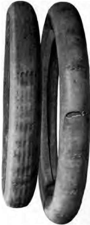
Ruined by tight chains. Observe where the metal cross pieces cut into the rubber at regular intervals. Chains should be applied with just play enough to creep.
