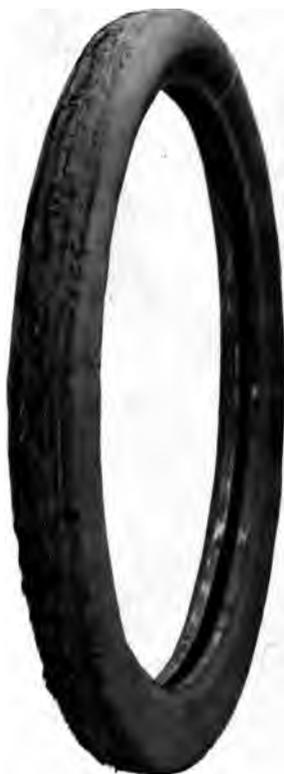
If the wheels do not run true the tire is scraped along. That wears down the tread, as you see here.
