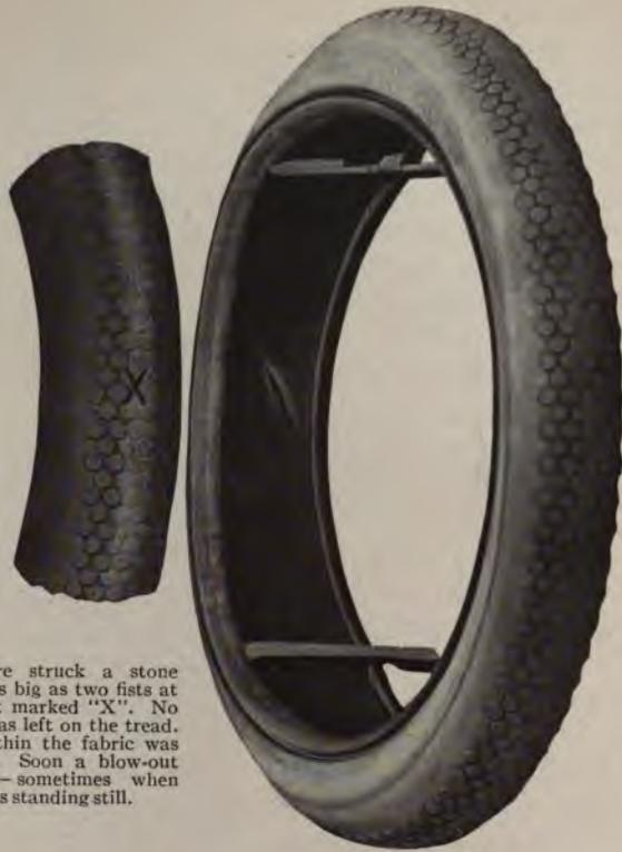
The tire struck a stone about as big as two fists at the spot marked "X". No mark was left on the tread. But within the fabric was broken. Soon a blow-out occurs — sometimes when the car is standing still.
