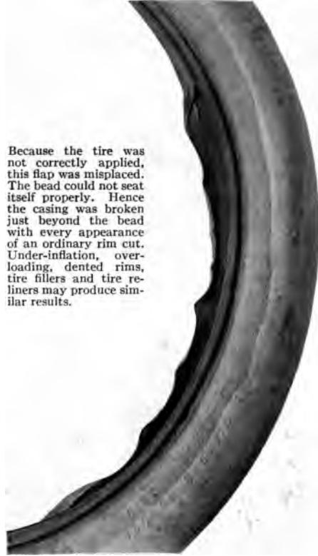
Because the tire was not correctly applied, this flap was misplaced. The bead could not seat itself properly. Hence the casing was broken just beyond the bead with every appearance of an ordinary rim cut. Under-inflation, overloading, dented rims, tire fillers and tire reliners may produce similar results.
