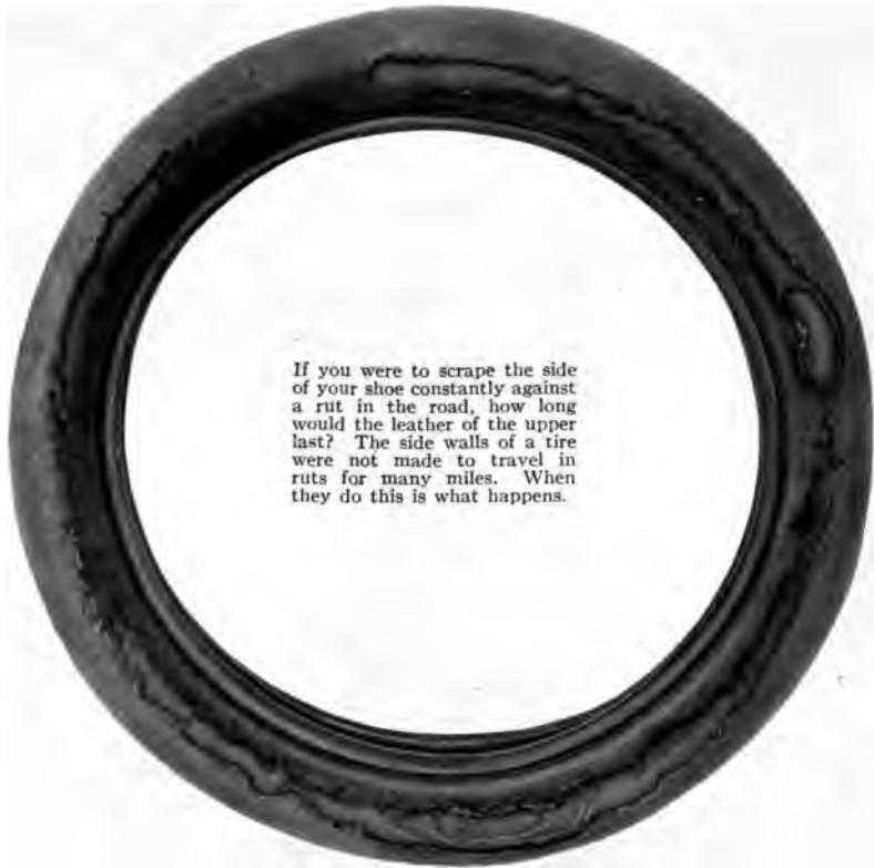
If you were to scrape the side of your shoe constantly against a rut in the road, how long would the leather of the upper last? The side walls of a tire were not made to travel in ruts for many miles. When they do this is what happens.
