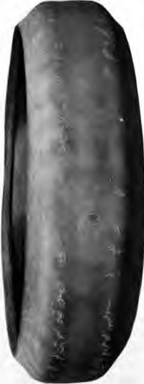
Here you see the effect of under-inflation or overloading. The tire has been turned inside out so as to expose the fabric. Note how the bending of the side walls, made possible by insufficient air-pressure, has broken the fabric.
