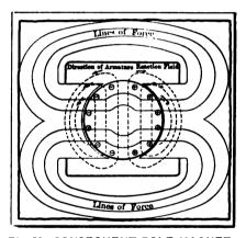
Fig. 50—CONSEQUENT POLE MAGNET, SHOWING LINES OF MAGNETIC FORCE AND ARMATURE REACTION
