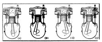
Fig. 3—SHOWING THE FOUR POSITIONS OF THE PISTON OF A MOTOR DURING THE FOUR-CYCLIC FUNCTIONS
