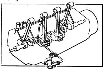
Fig. 88—FORCED FEED LUBRICATION DIAGRAM, SHOWING THE PUMP AND THE PIPING. THE OIL IS DRAWN FROM THE BASE AND IS FORCED BY THE PUMP THROUGH THE PIPES TO ALL THE BEARINGS
