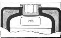
FIG. 24—SECTION OF A GASOLINE EN-GINE CYLINDER SO CONTRIVED THAT THE INTERNAL WALL IS CURVED AND THE EXTERIOR PRESENTS A FLATTENED APPEARANCE
