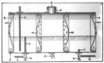
I Ig. 102—SECTION OF A GASOLINE TANK THAT CAN BE USED EITHER FOR PRESSURE OR GRAVITY FEED. THE TRANSVERSE SECTIONAL PLATES ARE TO PREVENT SWAYING OF THE LIQUID
