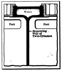
Fig. 25—SECTION OF THE PARTING WALL BETWEEN A PAIR OF CYL-INDERS SHOWING WATER IN THE INTERVENING SPACE
