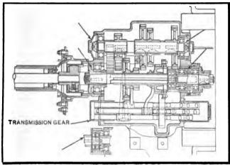
FIG. 60—SELECTIVE TYPE OF TRANSMISSION, SHOWING THE SELECTING ARMS AND UNIVERSAL JOINT AT REAR OF GEAR BOX
