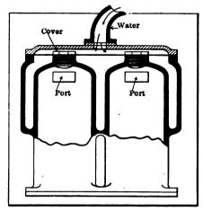
Fig. 31—PRESENTING A PAIR OF CYL-INDERS 80 DESIGNED THAT THE COVER MAY BE REMOVED IN ORDER TO GET AT AND SCRAPE SURFACES FREE OF DEPOSIT
