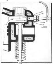
Fig. 28—SECTION OF A CYLINDER SHOWING HOW WATER IS CIRCU-LATED AROUND THE SPARK PLUG BOSS; THIS KEEPS THE SPARK PLUG FROM BURNING
