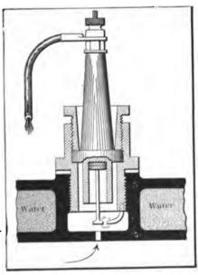
Fig. 74—SECTION OF A DEFECTIVE SPARK PLUG INDICATING AB-SENCE OF PACKING UNDER THE GLAND—PLUG WILL LEAK COMPRESSION
