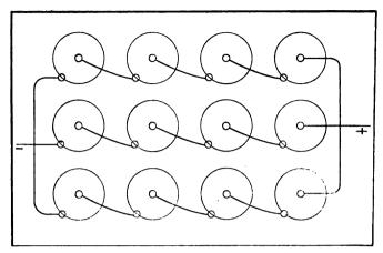
Fig. 36—DIAGRAM OF THREE SETS OF DRY CELLS CON-NECTED IN SERIES-PARALLEL
