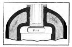
Fig. 21—SECTION OF A CYLINDER, 8HOWING A LARGE AMOUNT OF WATER OVER THE DOME OF THE COMBUSTION CHAMBER
