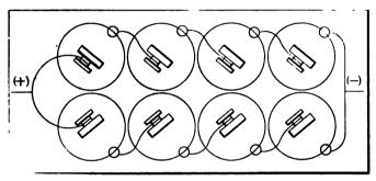
Fig. 35—DIAGRAM OF A SET OF DRY CELLS CONNECTED UP
