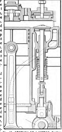
neto and the other Fig. 82—SECTION OF A MOTOR, SHOW-ING VALVE MECHANISM AND touching the motor. ADJUSTABLE PUSH RODS
