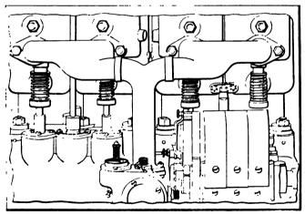
Fig. 17—DEPICTING THE CARBURETER NEAR THE MAGNETO AT THE SIDE OF A MOTOR; IT IS NECESSARY TO AVOID LEAKS OF GASOLINE IN ORDER NOT TO HAVE A FIRE HAZARD, DUE TO THE CLOSE PROXIMITY OF THE SPARKING EQUIPMENT
