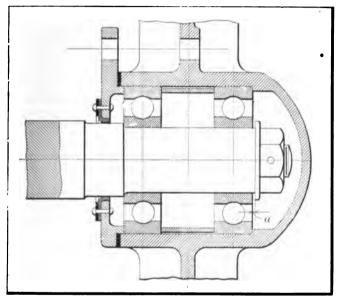
FIG. 67—SECTIONAL VIEW OF A SHAFT, SHOWING THE BALL
