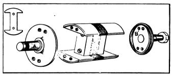
Fig. 49—BOBBIN ARMATURE FOR A CONVENTIONAL TYPE OF HIGH-TENSION MAGNETO
