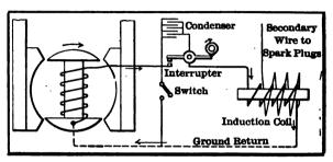
Fig. 53—DIAGRAM SHOWING THE PATH OF CURRENT IN A HIGH-TENSION MAGNETO SYSTEM WITH A SEPARATE INDUCTION COIL
