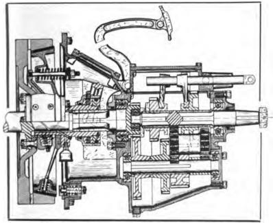
Fig. 63—LEATHER-FACED CLUTCH, WITH EXTERIOR SPRINGS ATTACHED TO A ROCKING SPIDER AND TRANS-MISSION GEARS WITH MILLED KEYWAY SHAFTS
