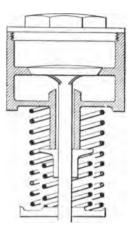
LEAK IN VALVE DUE TO WEAR IN THE GUIDES. THE IN-SERTED CAP AND **SPRING** EXTRA CAN BE USED FOR A TEM-PORARY RE-PAIR
