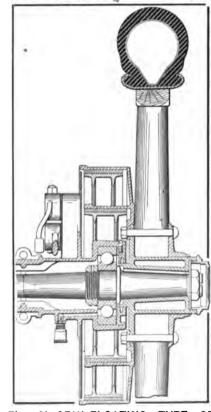
Fig. REAR AXLE IN WHICH THE WEIGHT CAR IS CARRIED BY THE LIVE AXLE
