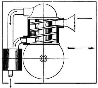
Fig. 87—METHOD OF PASSING THE AIR AROUND THE CYLIN-DERS TO OBTAIN EQUAL HEATING
