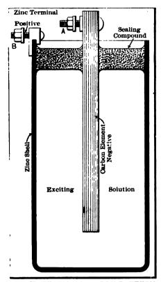
Fig. 37—SECTION OF A DRY BATTERY, SHOWING THE CARBON ELEC-TRODE IN THE CENTER AND THE ZINC CAN, WHICH ALSO SERVES AS THE OTHER (NEGATIVE) ELECTRODE
