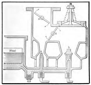
Fig. 11—SECTION OF A CARBURETER OF THE DOUBLENOZZLE TYPE WITH THE FLOAT LOCATED IN A BOWL
