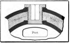
Fig. 22—SECTION OF A CYLINDER, 8HOWING THE PLUG IN THE HEAD 8O PLACED THAT IT IS LIKELY TO CAUSE A LEAK OF WATER INTO THE COMBUSTION CHAMBER
