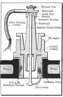
Fig. 73—SECTION OF A SPARK PLUG, SHOWING THE RELATIONS OF THE COMPONENTS
