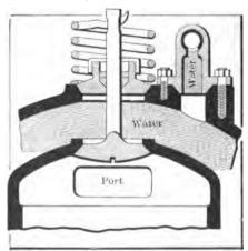
Fig. 20—SECTION OF A CYLINDER PRESENTING A METHOD OF KEEP-ING WATER OUT OF THE COMBUSTION CHAMBER, USING A GROUND-IN MUSHROOM ON A STEM, HELD TIGHT BY A SPRING
