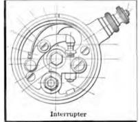
RUPTER WITH THE COVER OFF, SHOWING THE ROLLER CON-TACT MEMBER ON THE END OF THE SPRING-CON-TROLLED FINGER
