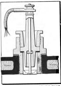
Fig. 78—SECTION OF A SPARK PLUG, SHOWING THE PROPER PLACING OF THE PACKING UNDER THE PORCELAIN AND CLEARANCE BETWEEN IT AND THE METAL PARTS
