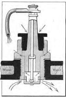
Fig. 77—SECTION OF A SPARK PLUG, SHOWING THE PORCELAIN IN CON-TACT WITH THE METAL WALL— THIS WILL CAUSE THE PLUG TO FAIL ELECTRICALLY; IN-SULATION TOO LOW
