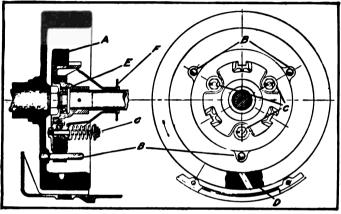
Fig. 58—ALTERNATE DISCS OF HARD COPPER AND STEEL SHOWN AT "A." COPPER DISCS DRIVEN FROM FLYWHEEL BY PINS "B." CLUTCH ACTUATION BY MEANS OF SPRINGS "C." CLUTCH CAN THROW NO END THRUST UPON CRANKSHAFT AS SAME IS TAKEN BY FRONT TRANSMISSION BEARING. CLUTCH HUB FLOATS UPON ANNULAR BEARING "E." FLANGE FOR BEARING OF CLUTCH THROW-OUT COLLAR AT "F."
