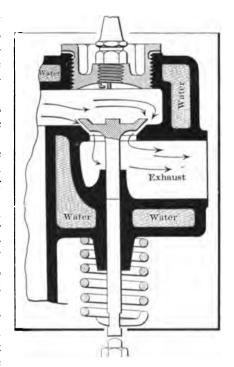
Fig. 95—LEAK. CAUSED BY THE BENDING OF THE EXHAUST VALVE STEM PREVENTING THE VALVE SEATING PROPERLY
