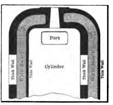
Fig. 27—SECTION OF A CYLINDER WITH A CORED HOLE IN THE DOME; THIS CORE MIGHT BE MISPLACED IN THE CASTING PROCESS AND A LEAK WOULD BE THE RESULT IN SERVICE
