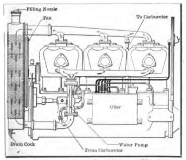
Fig. 98—SECTION OF THE WATER COOLING SYSTEM, SHOW-ING THE FLOW OF WATER WHERE A PUMP IS EMPLOYED
