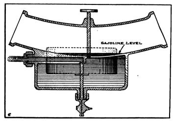
Fig. 12—SECTION OF THE DURYEA TYPE OF CARBURETER.
