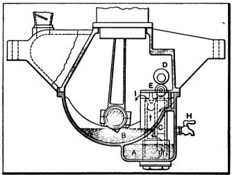
FIG. 70—PLUNGER TYPE OF LUBRICATOR PUMP DRIVEN BY A CAM ON THE CAMSHAFT. THE SCOOPS ON THE END OF THE CONNECTING RODS SPLASH THE OIL UP TO THE CYLINDERS AND WRIST PINS
