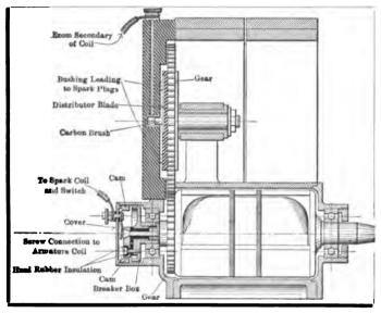
Fig. 80—SECTION OF A HIGH-TENSION MAGNETO, DEPICT-ING THE PROPER RELATIONS OF THE COMPONENTS, INDICATING COMPACTNESS; THE USE OF BALL BEARINGS, AND HOW THE PARTS ARE ASSEMBLED
