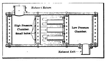
Fig. 83—SECTIONAL VIEW OF A MUFFLER (EXHAUST BOX), SHOWING THE TRAVEL OF THE GASES
