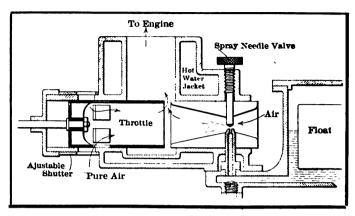
Fig. 14—DEPICTING A TYPE OF CARBURETER USING A SLEEVE-VALVE IN THE AUXILIARY AIR-PASSAGEWAY, SHOWING THE GASOLINE NOZZLE TO THE SIDE OF THE FLOAT-BOWL JUST AT THE JUNCTION OF THE TRANSFER PORT THROUGH WHICH THE MIXTURE GOES TO THE COMBUSTION CHAMBER OF THE MOTOR
