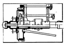
Fig. 65—SHOWING DISPOSITION OF IN-TERNAL AND EXTERNAL EXPAN-SION BRAKES ON THE REAR WHEEL HUB
