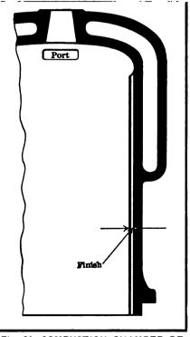
Fig. 91—COMBUSTION CHAMBER DE-SIGNED TO ALLOW THE PISTON RINGS TO OVERLAP
