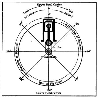
Fig. 72—DIAGRAMMATIC SCHEME, SHOWING THE RELA TIONS OF THE MARKINGS ON THE FLYWHEEL OF A MOTOR WITH RESPECT TO THE POSITION OF THE PISTON
