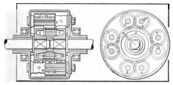
FIG. 61—TYPE OF DIFFERENTIAL GEAR USING SQUARE-CUT TEETH IN EACH PINION
