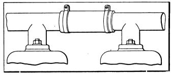
FIG. 101—A BROKEN GASOLINE PIPE CAN TEMPORARILY BE REPAIRED IN A SIMILAR MANNER TO THAT USED IN JOINING WATER PIPING
