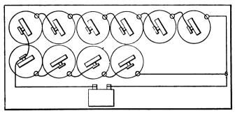
Fig. 39—DIAGRAM OF A SYSTEM OF DRY CELLS PROPERLY CONNECTED UP
