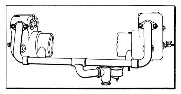
FIG. 16—SCHEME OF LOCATING THE CARBURETER MIDWAY
