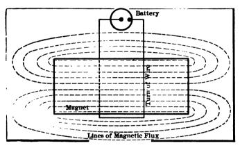
Fig. 58—MAGNETIC DIAGRAM OF A SPARK COIL, SHOWING HOW THE LINES OF FORCE THREAD THE WIRE\*
