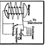
FIG. 55—SHOWING THE RE-LATION OF THE CONDENS-ER TO THE INTERRUPT-ER; THE CONDENSER BEING IN PARALLEL ACROSS THE GAP
