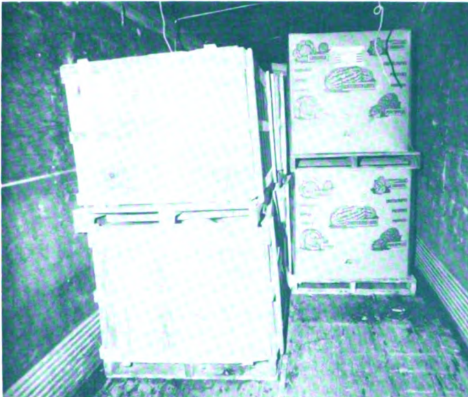
Figure 3.—Type 3 bin (right) and type 4 bin (left) in trailer during unloading at destination warehouse.
