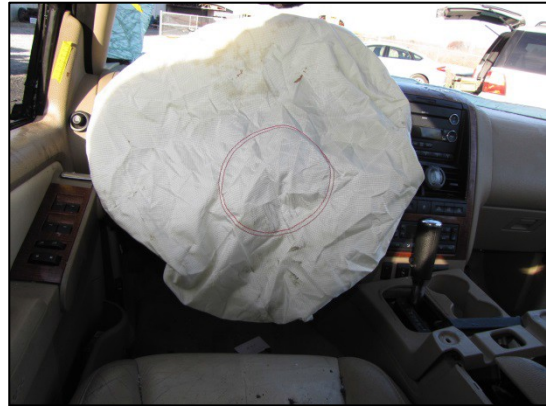
Figure 22: Image depicting the deployed drive air bag in the Ford.
