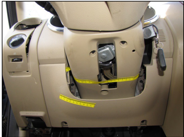
Figure 21: Interior image of the Ford depicting the driver contact to the left instrument panel and knee bolster.
