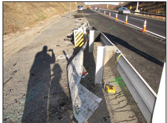
Figure 16: East-facing image of the extruded W-beam flattened by the Ford as it struck the ground near its final rest position.
