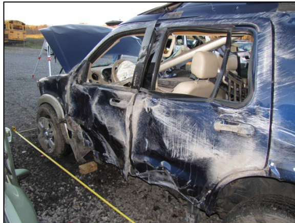
Figure 19: Oblique view of the damage to the Ford's left plane.
