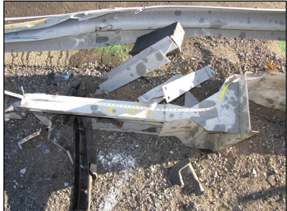
Figure 14: Overhead view depicting the bumper reinforcement bar in the displaced end terminal.
