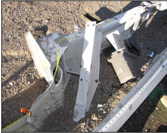
Figure 10: Northeast-facing image of Post 1, which remained attached to the displaced end terminal.
