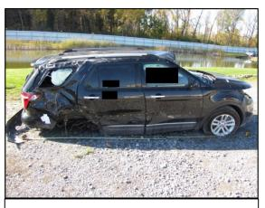
Figure 10: Right side view of the Ford depicting the impact damage associated with Event 1.
