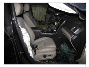
Figure 13: Right interior view of the Ford's front row right seat.
