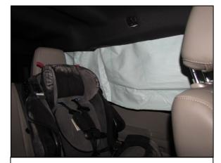
Figure 16: Interior view of the Ford depicting the deployed left IC air bag at the second row left posi-
