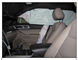
Figure 15: Interior view of the Ford depicting the deployed air bags at the front row right position.
