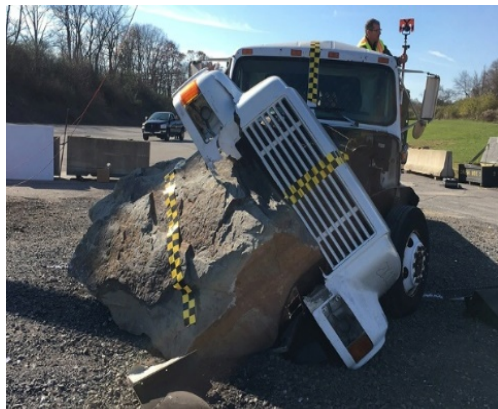
Figure 4. Photo. Example of passive, improvised, or landscape VSB used to stop a heavy vehicle.
