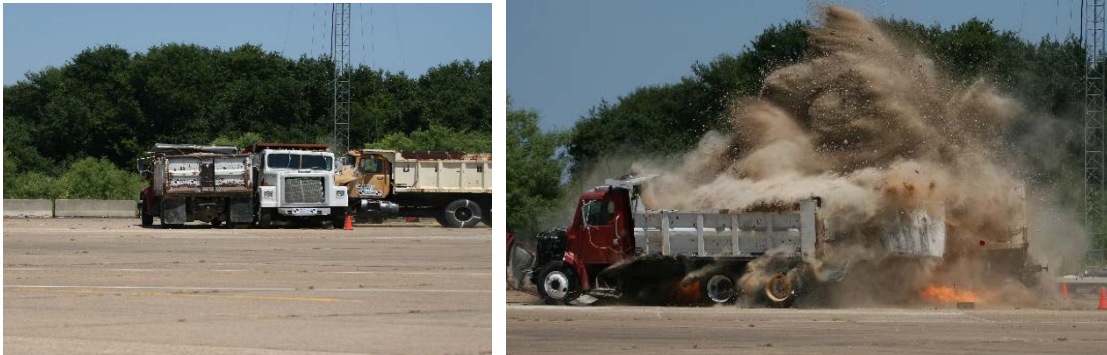
Figure 37. Photos. Two dual-axle highway vehicle barrier heavy goods truck performance test.
