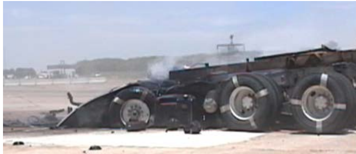
Figure 40. Photo. Heavy goods truck post-impact with K12 active wedge VSB.
