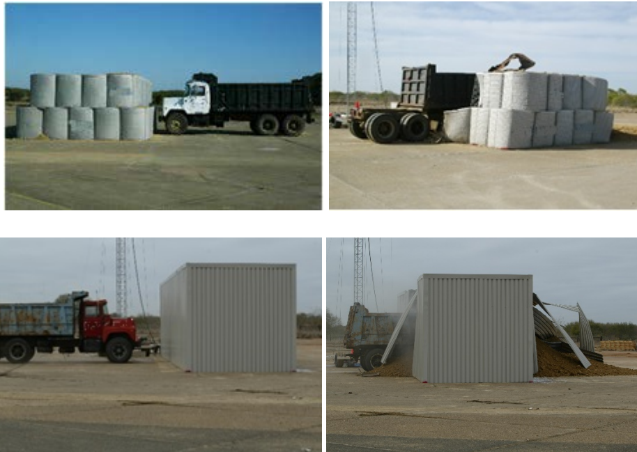
Figure 25. Photos. Earth-filled barriers versus heavy goods truck performance test.
