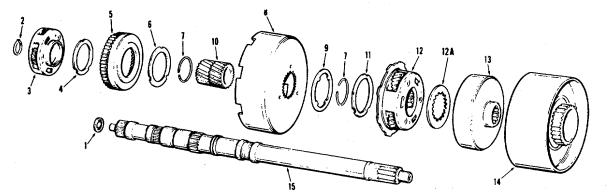
Figure 6-41. Output Shaft and Gear Train
