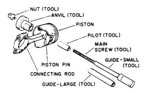
Figure 5-2. Tool Arrangement For Removing Piston Pin
