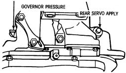
Figure 5-19. Pressure Test Locations (Rear End of Transmission)
