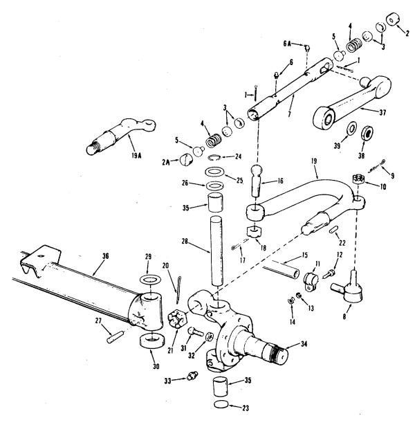
Figure 6-19. Front Axle and Drag Link Group
