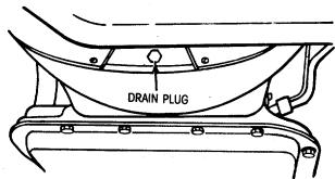
Figure 5-7. Drain Plug Location
