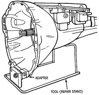
Figure 5-9. Transmission Installed on Control Stand
