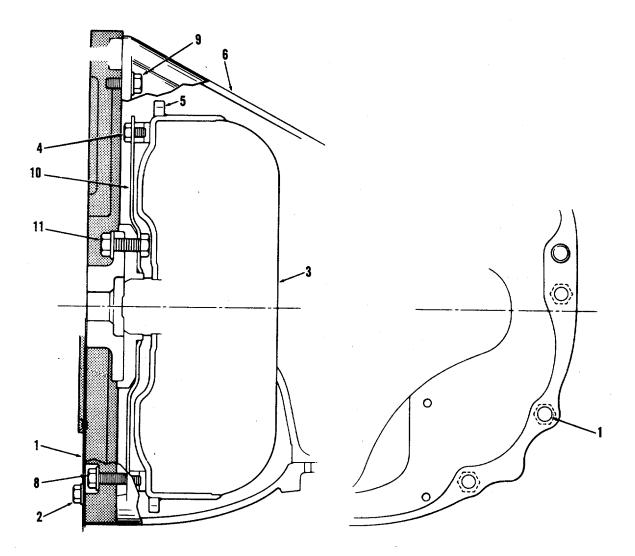
Figure 6-29. Transmission and Torque Converter
