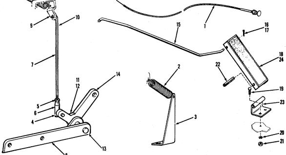
Figure 6-8. Accelerator Linkage Group
