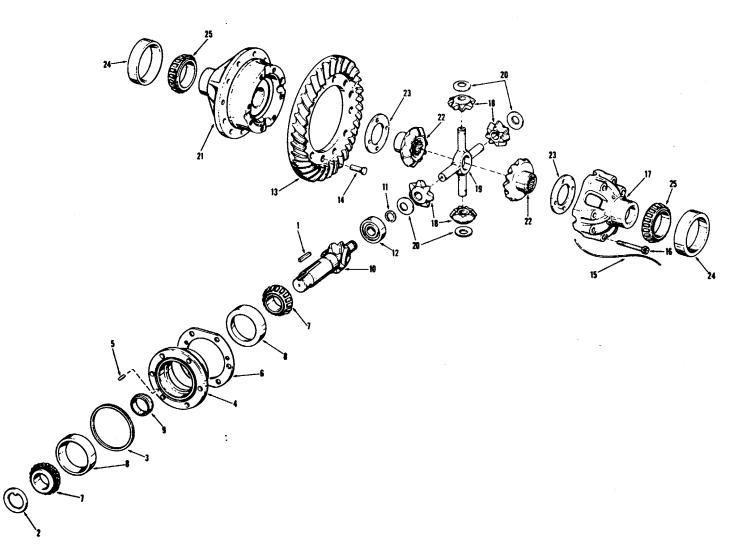
Figure 6-25. Differential and Carrier Assembly
