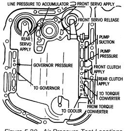
Figure 5-20. Air Pressure Test Locations 5-32
