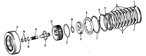
Figure 6-40. Rear Clutch Assembly
