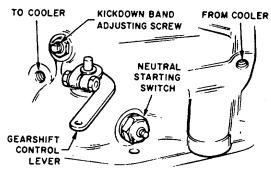
Figure 5-8. Location of Gearshift Control Lever NOTE
