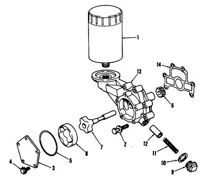
Figure 6-12. Engine Oil Pump and Filter Assembly
