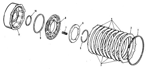
Figure 6-39. Front Clutch Assembly
