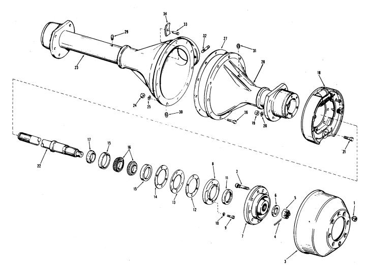
Figure 6-26. Rear Axle and Housing
