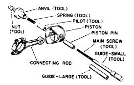
Figure 5-5. Tool Arrangement for Installing Piston Pin
