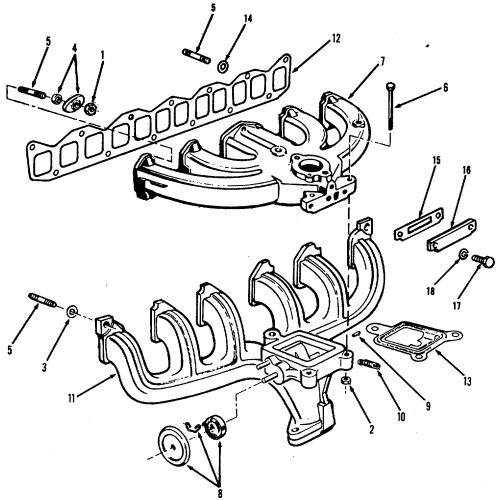
Figure 6-11. Engine Manifold Group
