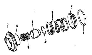
Figure 6-34. Low and Reverse Servo Assembly
