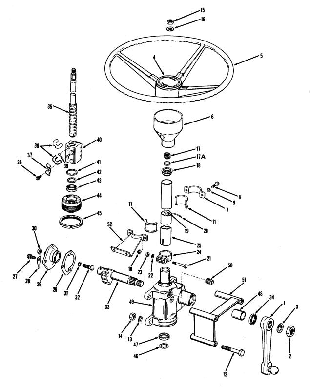
Figure 6-17. Steering Gear Group
