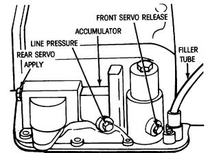
Figure 5-18. Pressure Test Locations (Right Side of Transmission) 5-31
