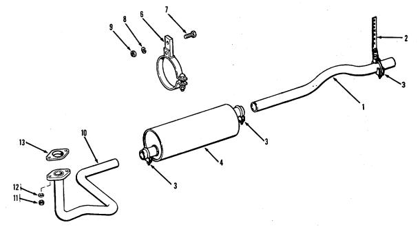
Figure 6-10. Exhaust and Muffler Group
