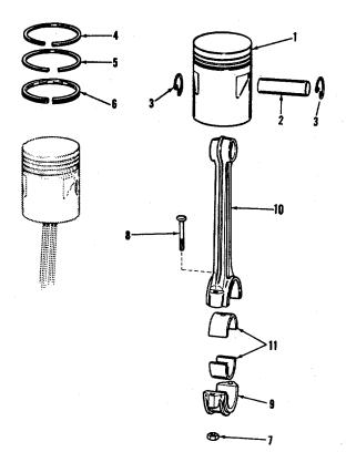
Figure 6-15. Piston and Connecting Rod Group
