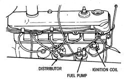
Figure 1-3. Right Side View of Engine
