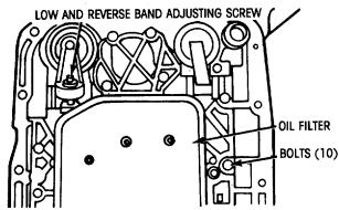
Figure 5-17. Bottom View of Transmission (Pan Removed)
