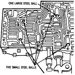
Figure 5-12. Steel Ball Location
