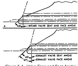
Figure 5-4. Valve Face and Seat Angles
