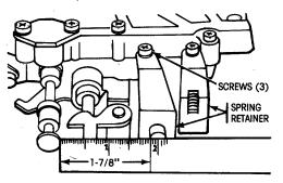
Figure 5-13. Measuring Spring Retainer Location
