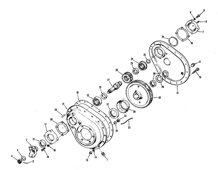
Figure 6-24. Rear Axle Drop Gear Case
