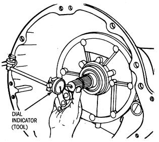
Figure 5-10. Measuring Drive End Plug
