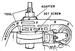
Figure 5-11. Location of Overrunning Clutch Cam
