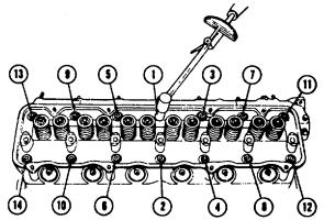
Figure 5-6. Cylinder Head Bolt Tightening Sequence
