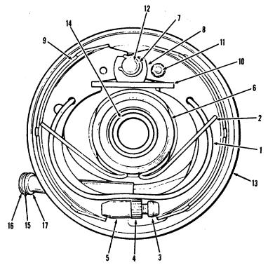
Figure 6-43. Parking Brake Assembly
