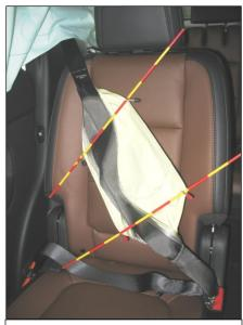
**Figure 18:** Second row right inflatable safety belt air bag within the Ford.
