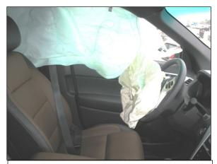
**Figure 10:** Deployed air bag systems within the front left seating position of the Ford.
