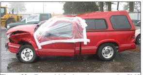
**Figure 22:** Forward left plane damage to the GMC from the Event 1 impact.
