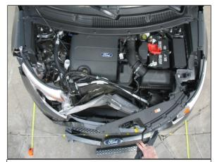
**Figure 5:** Overhead view of the Event 1 frontal damage sustained by the Ford (*note bumper beam deformation*).
