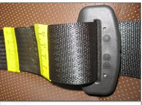
Figure 9: Latch plate and safety belt webbing loading from the Ford's front right passenger.
