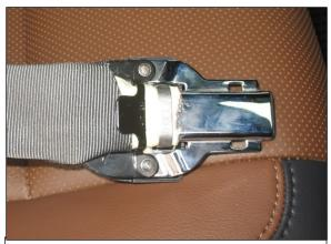
**Figure 12:** Top view of the inflatable safety belt latch plate within the Ford.
