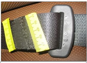
Figure 8: Loading evidence on the driver's safety belt webbing and latch plate within the Ford.
