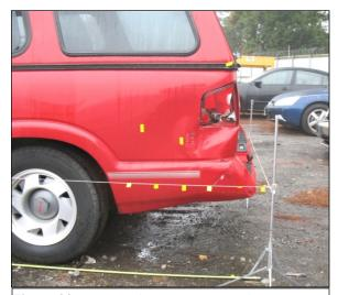
**Figure 23:** Event 2 damage pattern to the rear aspect of the GMC's left plane.
