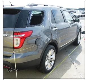
**Figure 7:** Event 2 damage pattern to the right plane of the Ford.
