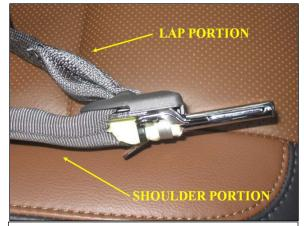
Figure 14: Lateral view of the inflatable safety belt latch plate within the Ford.
