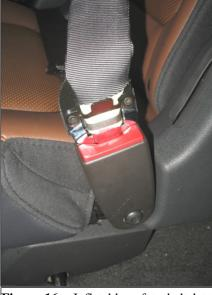
**Figure 16:** Inflatable safety belt latch plate engaged in buckle within the Ford.
