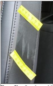
Figure 20: Second row left loading evidence within the Ford.
