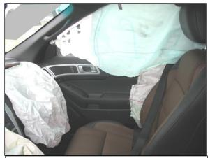
Figure 11: Deployed air bag systems within the front right seating position of the Ford.
