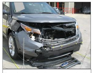
Figure 6: Frontal plane damage pattern and residual crush profile to the Ford from the Event 1 impact.
