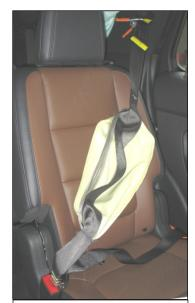
Figure 19: The Ford's second row left inflatable safety belt.
