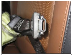
**Figure 15:** Compressed gas delivery tube within the Ford's inflatable safety belt latch plate.
