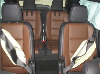
Figure 17: Deployed second row inflatable safety belts within the Ford at the time of SCI inspection.
