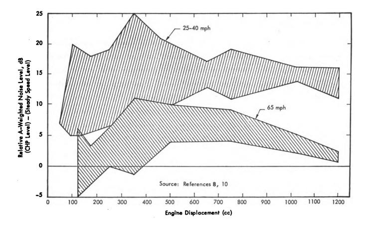
Figure 5. Difference Between CHP Method Acceleration and Steady Speed Noise Levels for 1973 Model Motorcycles
