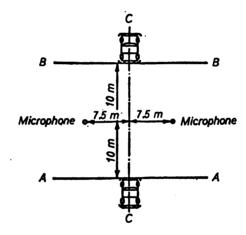
Fig. 1. - Measuring positions for measurement with vohicles in motion
