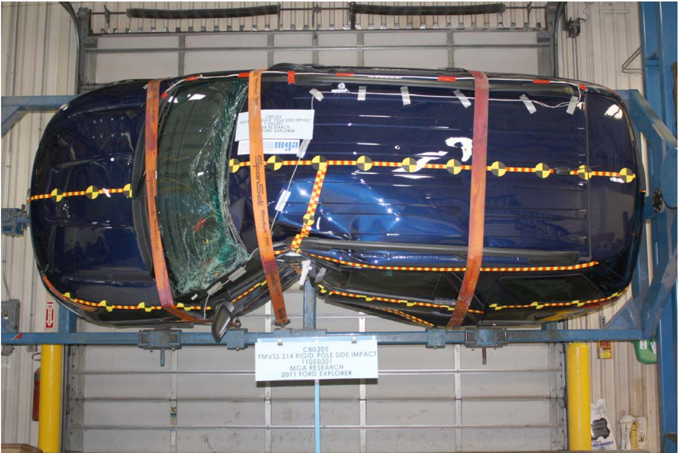
Post-Test Vehicle at 270 Degree Rollover
