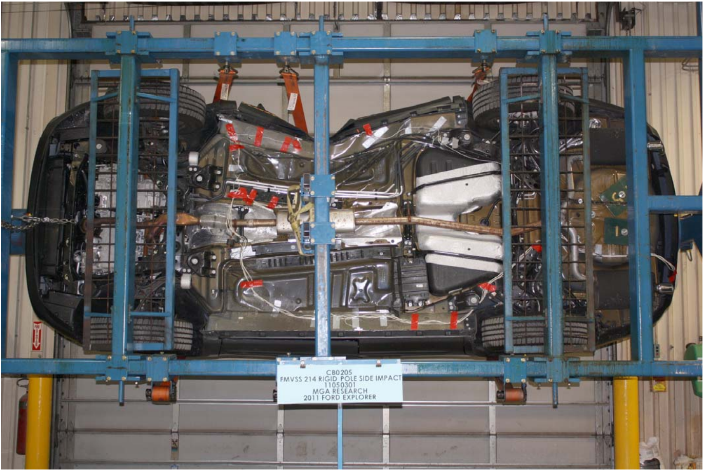
Post-Test Vehicle at 90 Degree Rollover
