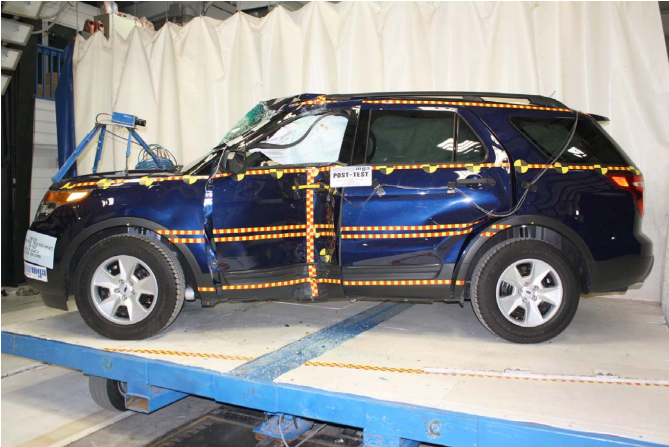
Post-Test Impacted Side View of Test Vehicle
