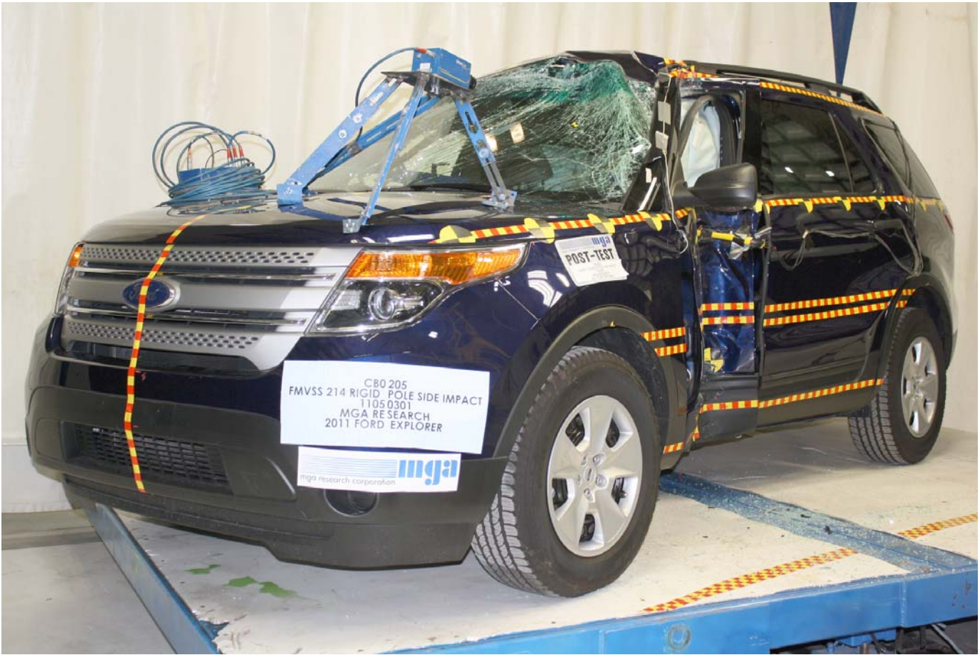
Post-Test \frac{3}{4} Front View of Impact Zone
