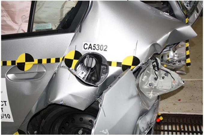
Figure A-57: Post-Test Fuel Filler Cap View
