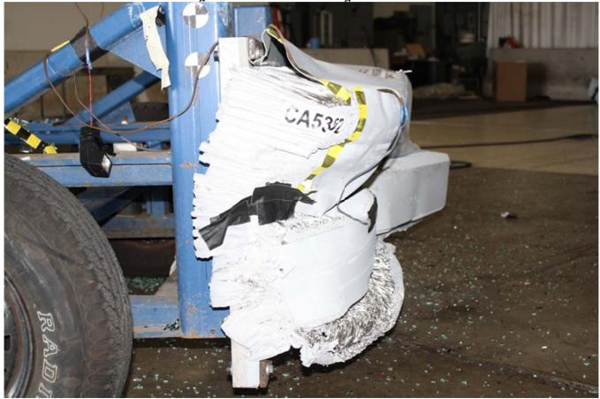
Figure A-28: Post-Test MDB Right Side View
