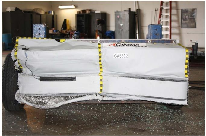
Figure A-24: Post-Test MDB Front View
