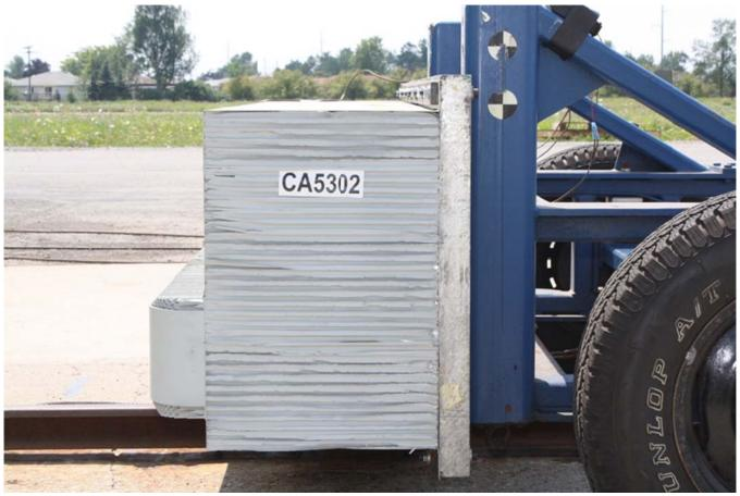
Figure A-25: Pre-Test MDB Left Side View
