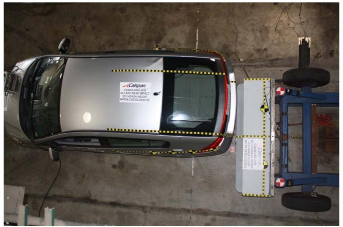
Figure A-31: Pre-Test Overhead Vehicle and MDB View
