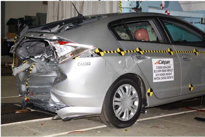
Figure A-20: Post-Test Right Rear Three-Quarter View
