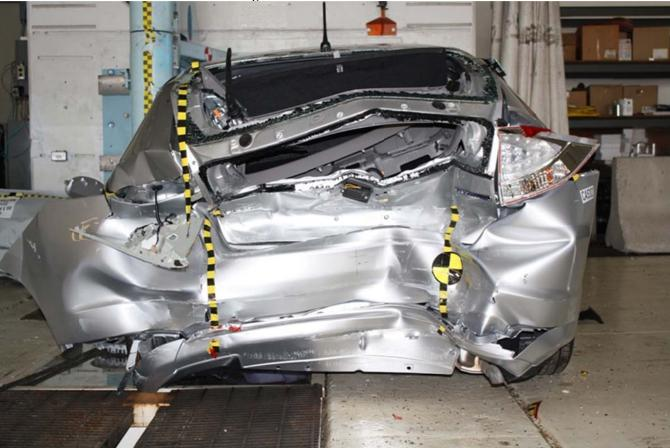
Figure A-22: Post-Test Rear View
