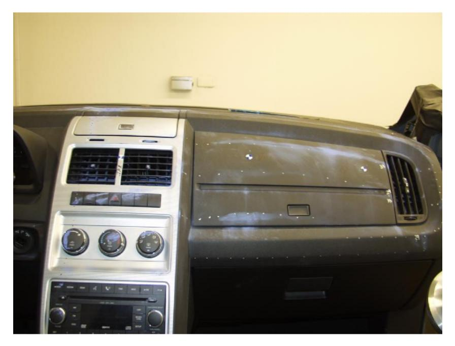
Figure A-14: DELINEATED INSTRUMENT PANEL IMPACT ZONE POST-TEST
