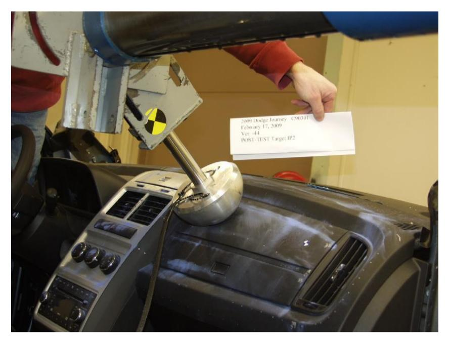
Figure A-18: INSTRUMENT PANEL IMPACT #2 POST-TEST
