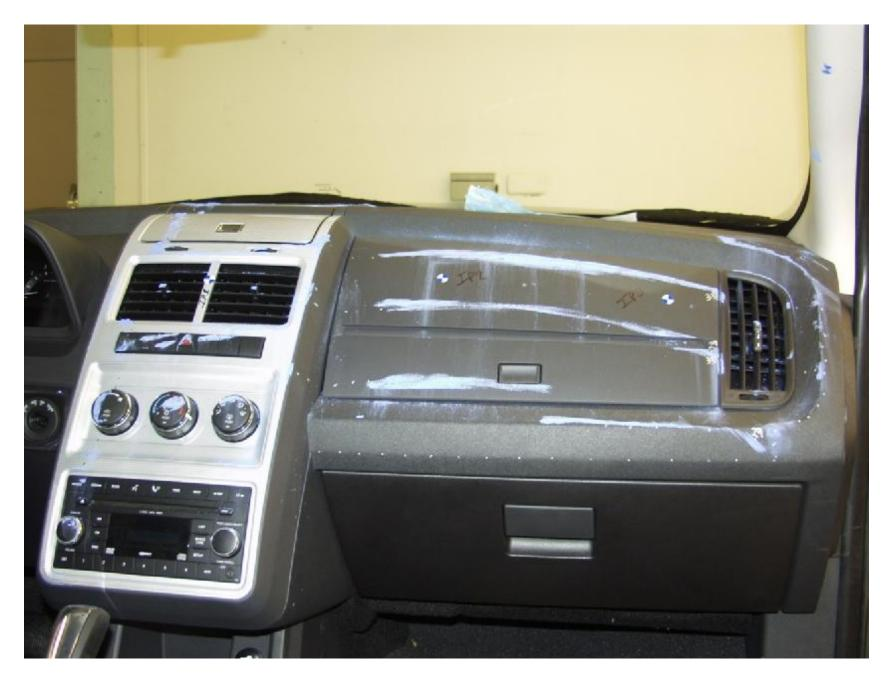
Figure A-13: DELINEATED INSTRUMENT PANEL IMPACT ZONE PRE-TEST
