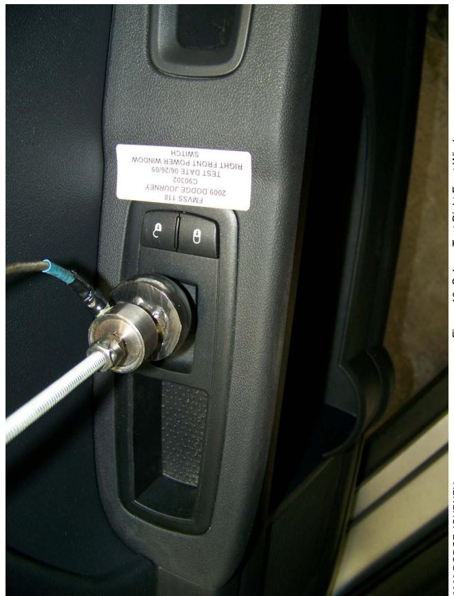
Figure 13: Sphere Test Right Front Window
