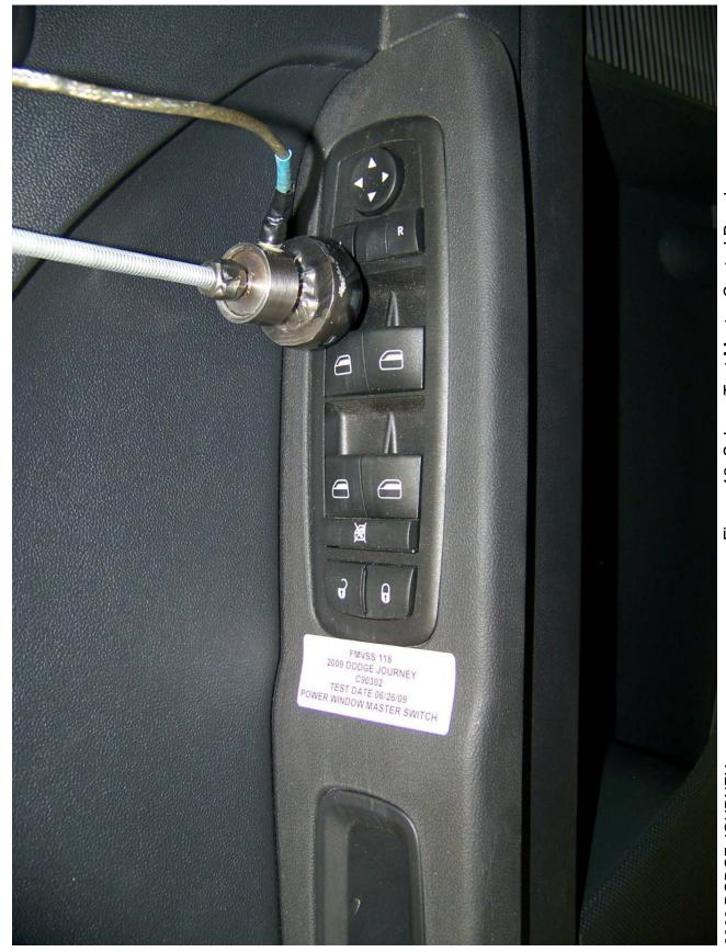
Figure 12: Sphere Test Master Control Panel
