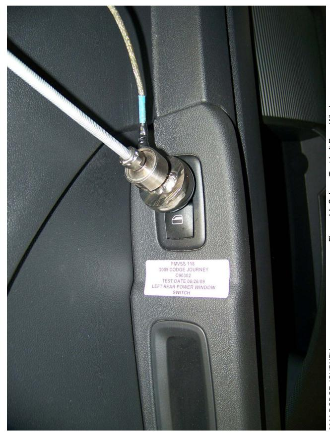
Figure 14: Sphere Test Left Rear Window
