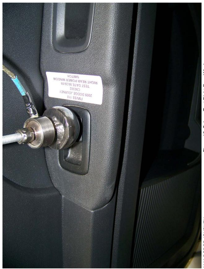
Figure 15: Sphere Test Right Rear Window
