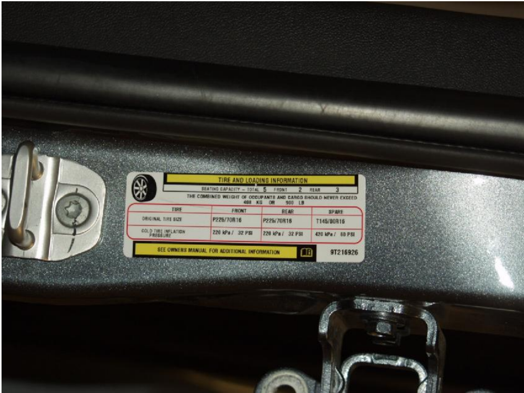
Figure A-6 : VEHICLE'S TIRE INFORMATION LABEL
