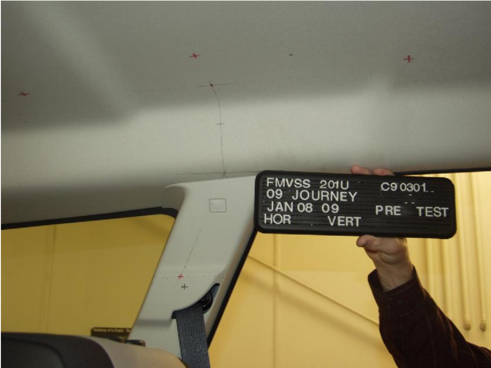
Figure A-11 : PRE-TEST DRIVER SIDE OTHER PILLAR
