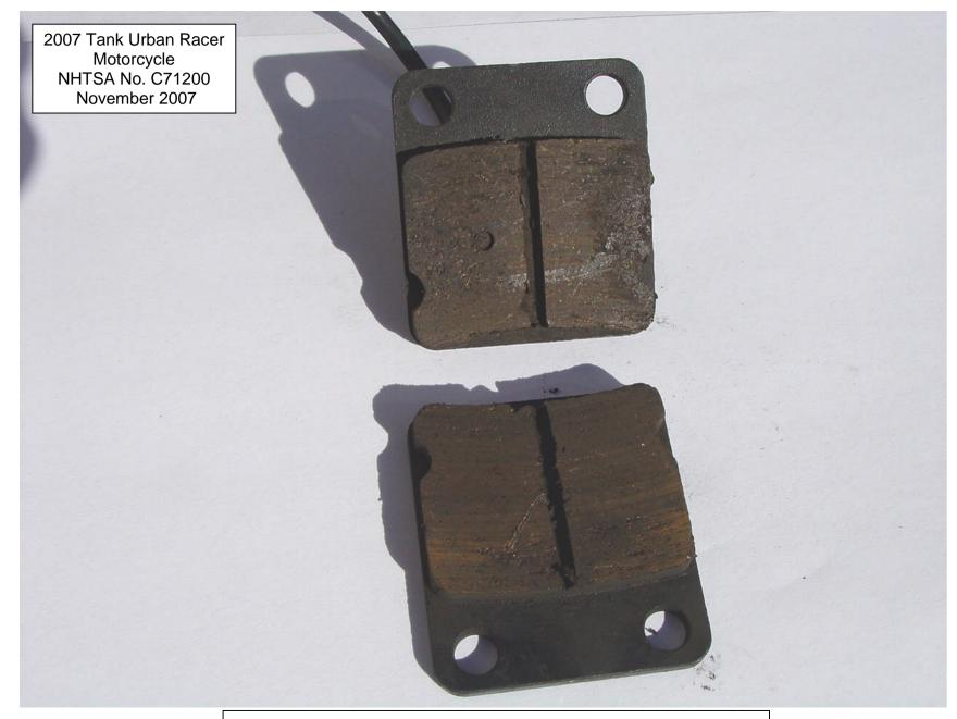
Condition, Front Brake Linings – Post Test
