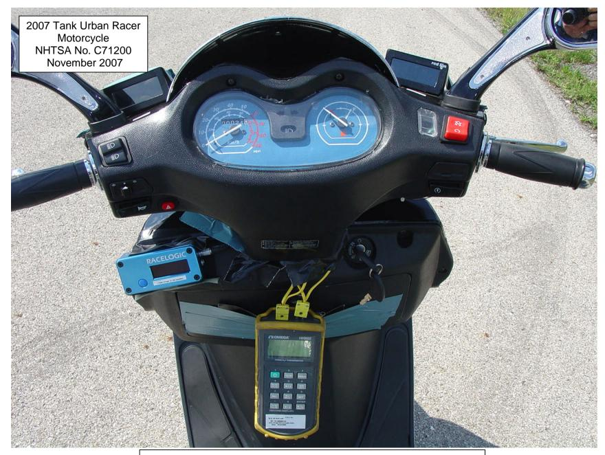
Instrumentation Installed on Vehicle
