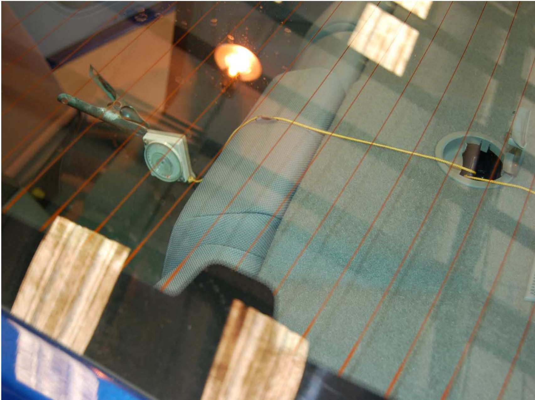
FIGURE 5.14 ROW 2, LEFT SIDE TOP TETHER ROUTING
