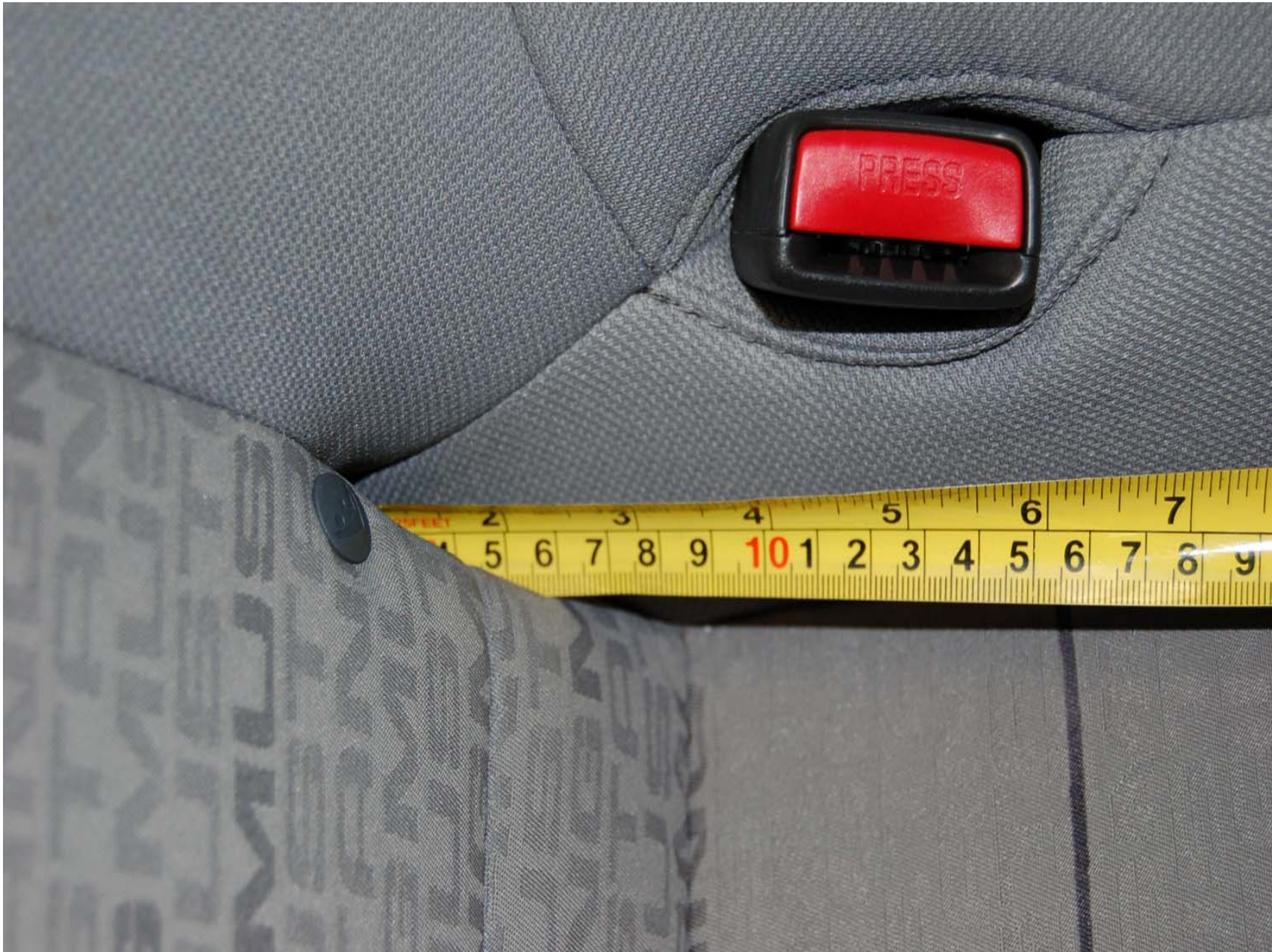
FIGURE 5.28 ROW 2, RIGHT SIDE INBOARD SRP MEASUREMENT
