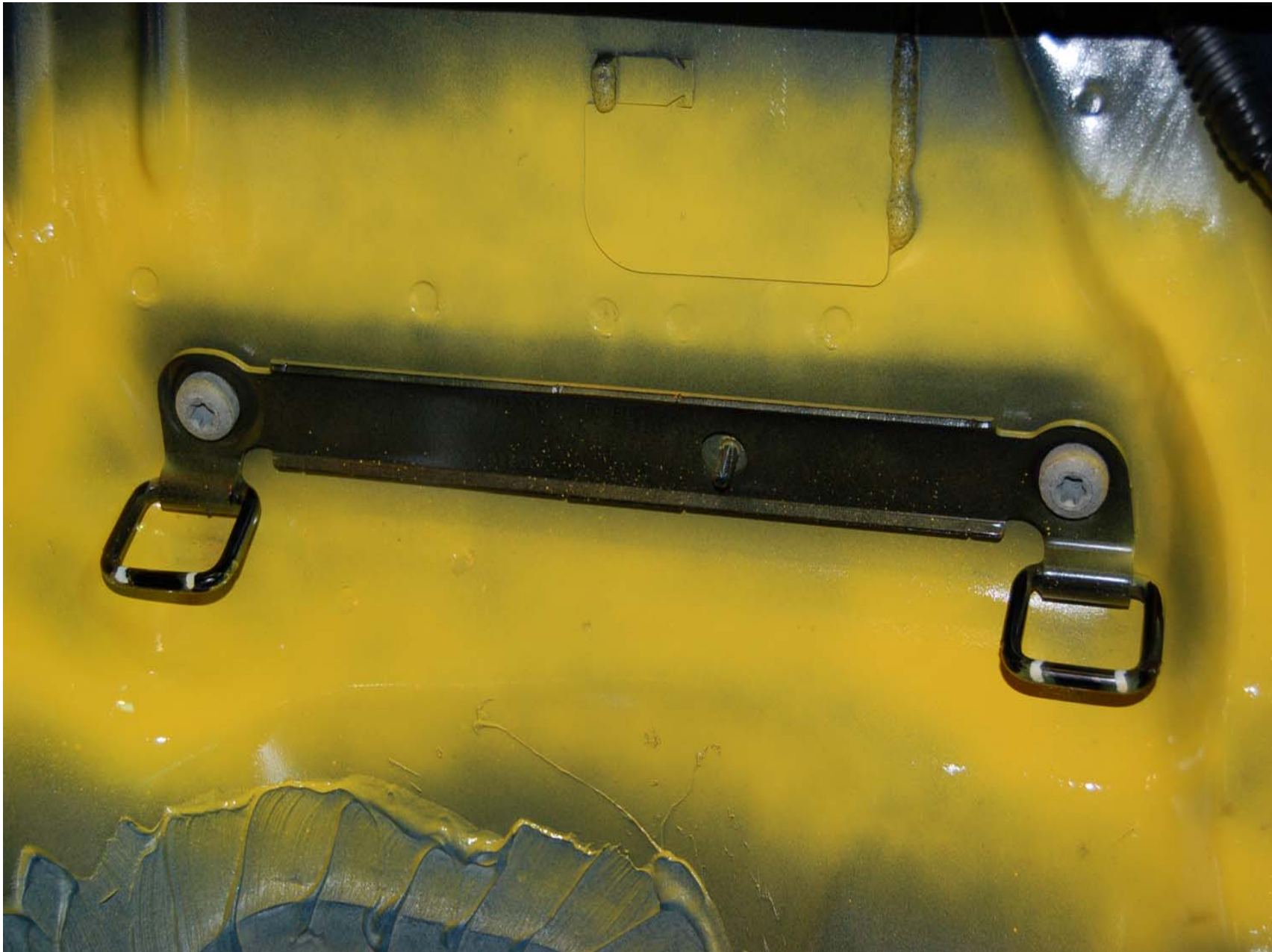
FIGURE 5.7 ROW 2, LEFT SIDE LOWER ANCHORS, PRE-TEST
