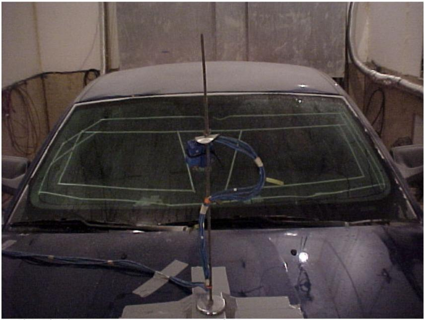
FIGURE 5.10 DEFROSTED AREA AT 20 MINUTES TEST #1
