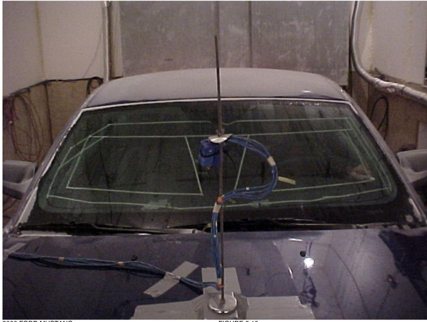
FIGURE 5.13 DEFROSTED AREA AT 20 MINUTES TEST #2
