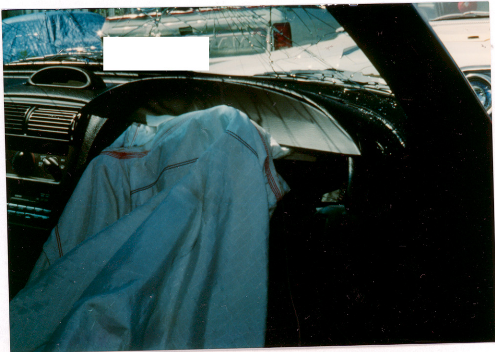
14. Close-up view of the passenger side air bag module.
