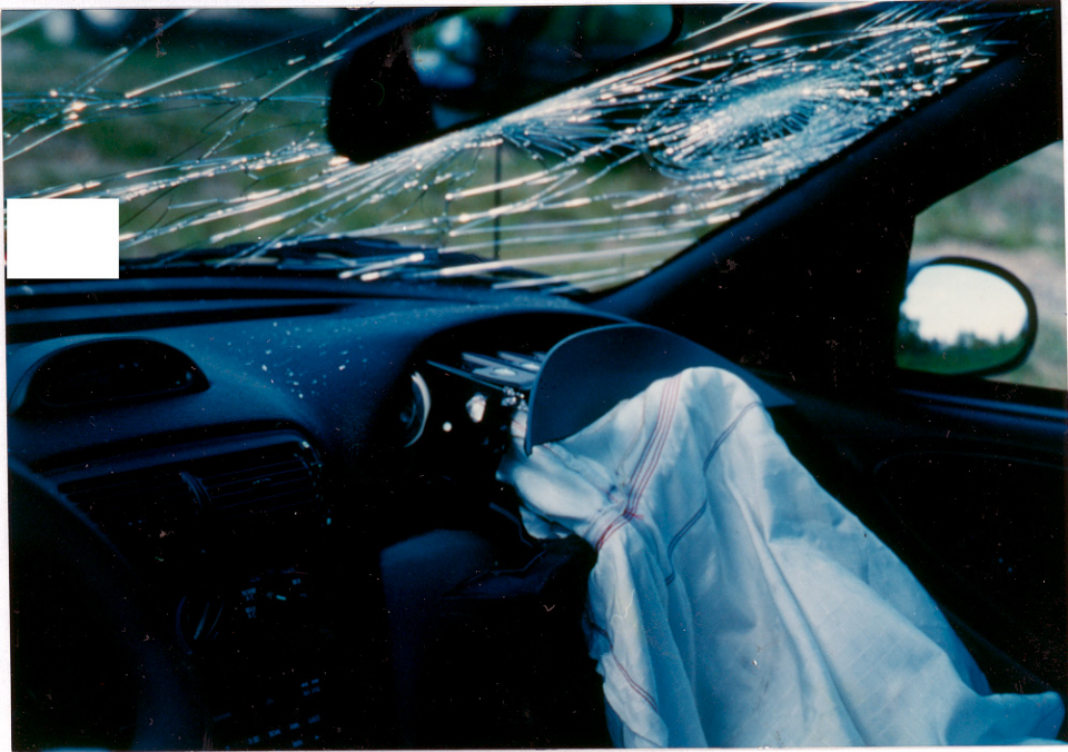
13. Rearward displacement/separation of the passenger side air bag module.
