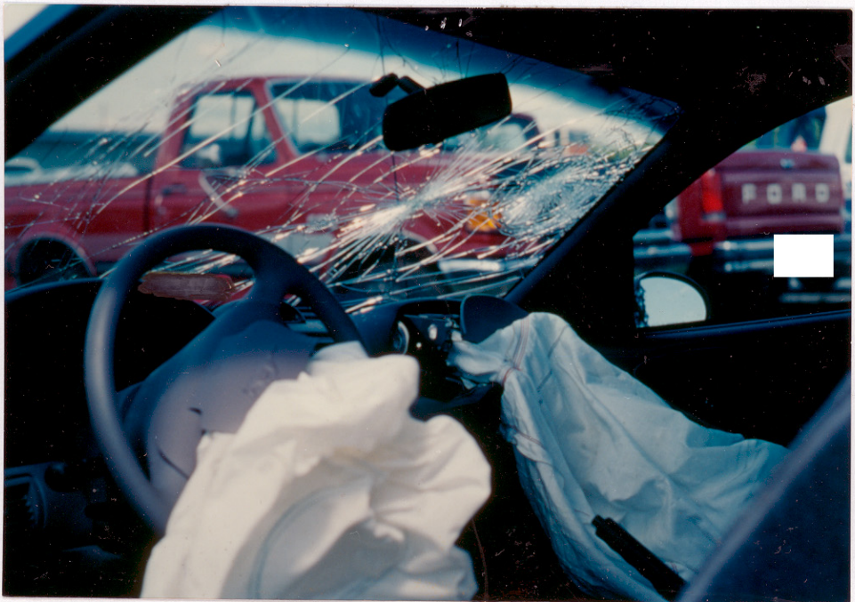
12. Overall interior view of the deployed air bags and windshield contacts.
