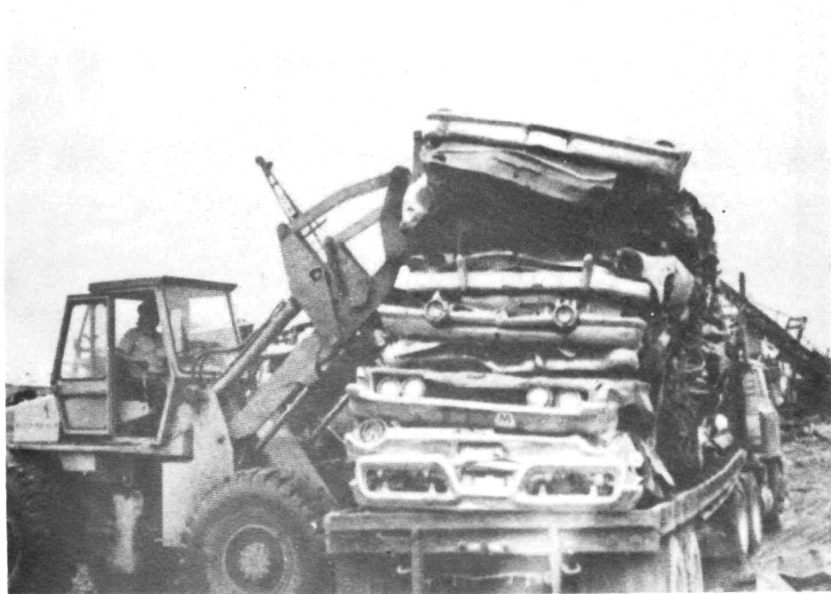
CRUSHED VEHICLES, APPROXIMATELY 20, BEING LOADED FOR TRIP TO METAL SHREDDER AND FURTHER PROCESSING-RECYCLING. U.S. STEEL PRODUCTION CONTAINS 55% SCRAP AT PRESENT.
