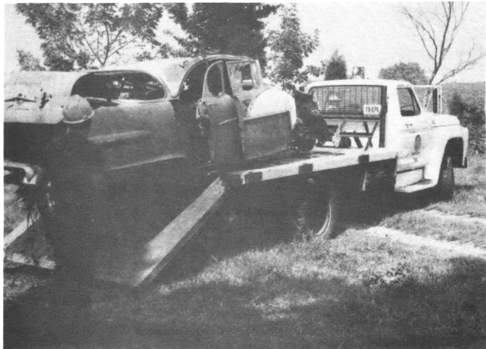
THIS VEHICLE IS AMOST LOADED, WINCH IS MOUNTED BEHIND TRUCK CAB. CHAIN WITH LOAD BINDER ARE USED TO SECURE VEHICLE AFTER LOADING. CAB PROTECTOR AND LOADING RAMP EASILY SEEN ALSO FROM THIS VIEW.
