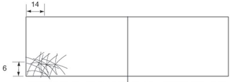
Windshield cracked on left due to contact by rear hood edge
