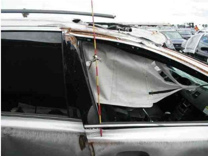
B PILLER DAMAGE
