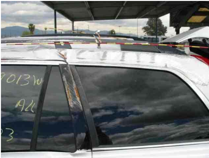
UPPER DAMAGE B TO C PILLER (ID=210206481)
