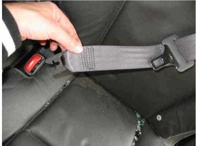
LEFT SEAT BELT LOWER FASTENER (ID=210206592) DISCONNECTED / PSB
