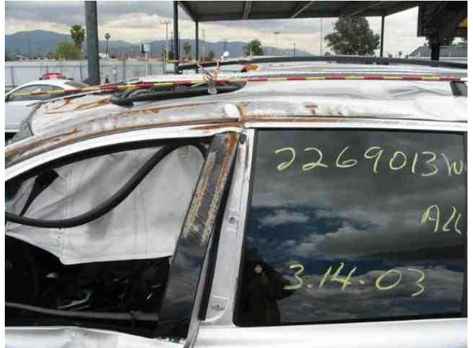
UPPER DAMAGE A TO B PILLER (ID=210206482)
