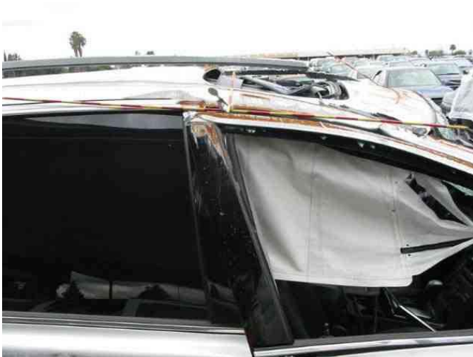
UPPER DAMAGE A TO B PILLER
