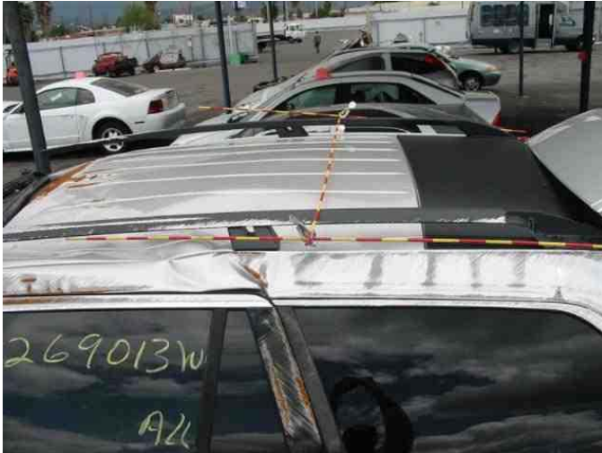
UPPER DAMAGE B PILLER AREA (ID=210206480)
