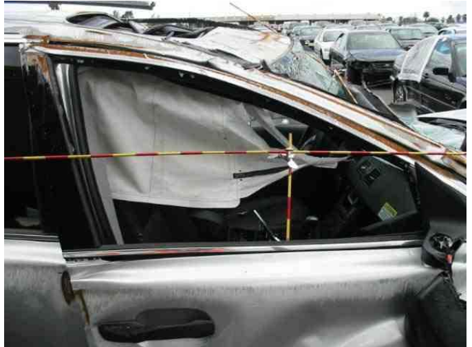
RIGHT FRONT DOOR AREA DAMAGE (ID=210206490)
