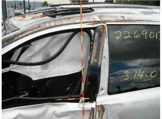
B PILLER DAMAGE
