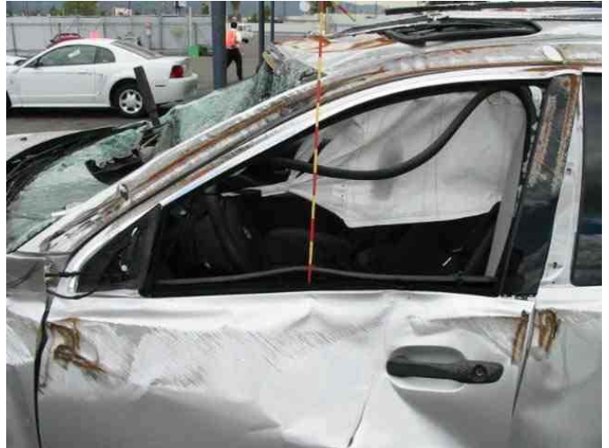
LEFT FRONT DOOR DAMAGE AREA (ID=210206494) MID
