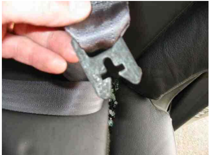
LEFT SEAT BELT LOWER FASTENER (ID=210206589) REMOVED
