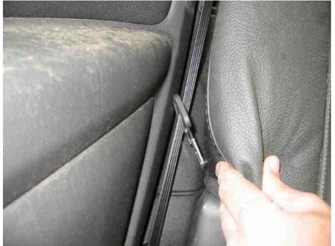
RIGHT PRETENSIONER DEPLOYED
