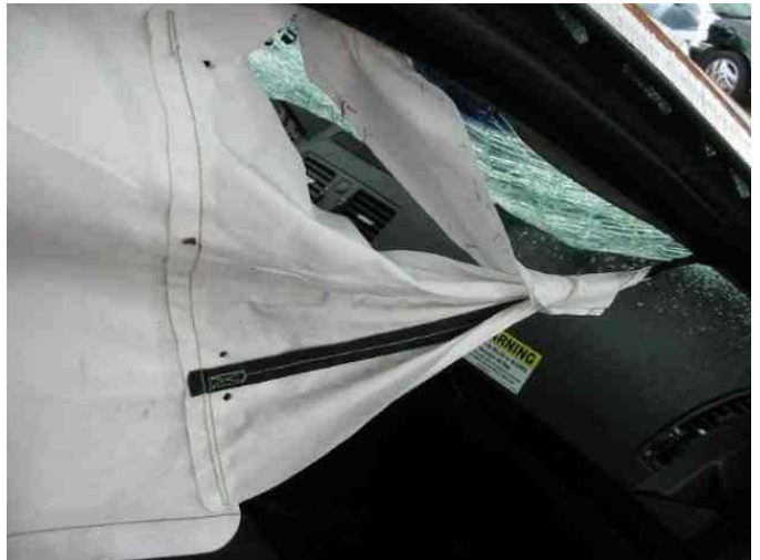
LOOKING IN TO RIGHT FRONT TETHER (ID=210206620)
