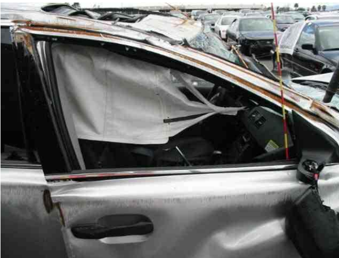
RIGHT FRONT DOOR AREA DAMAGE (ID=210206489) FRONT
