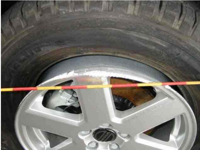
DAMAGE TO LEFT REAR WHEEL (ID=21020666)
