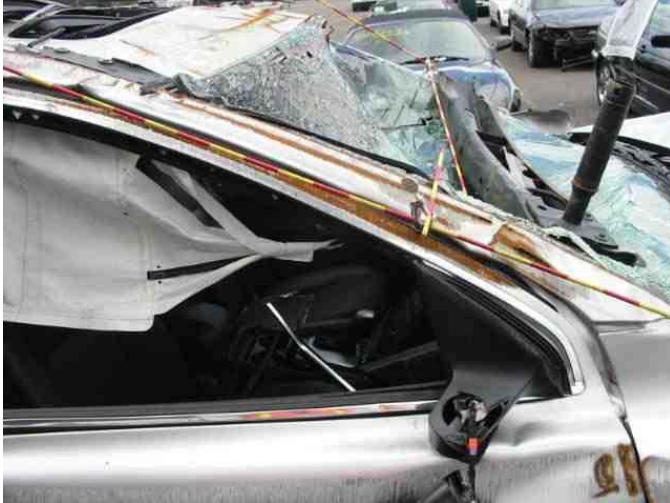
A PILLER DAMAGE
