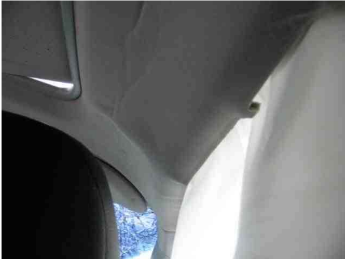
UPPER CURTAIN COMING OUT OF ROOF (ID=210206558)
