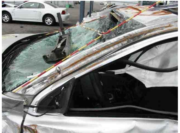
A PILLER DAMAGE (ID=210206483)
