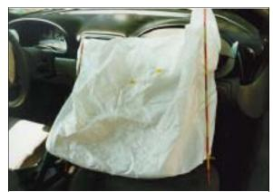
**Figure 8:** Case vehicle's deployed front right passenger air bag; Note: yellow tape indicates occupant contact points (case photo #50)
