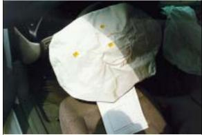
**Figure 7:** Case vehicle's deployed driver air bag; Note: yellow tape indicates occupant contact points (case photo #47)
