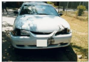
**Figure 5:** Case vehicle's damaged front end showing torn off bumper fascia placed back onto reinforcement bar (case photo #16)
