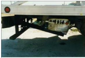
**Figure 4:** Close-up of Ford truck's damaged right rear showing primary damage to undercarriage; Note: yellow dot indicates forward-most point of direct damage (case photo #60)
