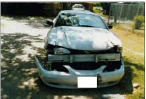
**Figure 2:** Case vehicle's frontal damage; Note: torn-off front bumper fascia and reinforcement bar (case photo #13)
