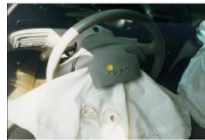
**Figure 6:** Case vehicle driver air bag module's top cover flap showing (i.e., yellow tape) scratch near flap's logo and vent ports (case photo #46)
