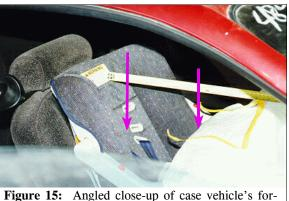
Figure 15: Angled close-up of case vehicle's forward facing child safety seat secured in front right seating position showing close proximity [8 cm (3.1 in)-between arrows] of skin transfer (i.e., taped area) on front portion of air bag in relation to center of safety seat's back (case photo #35)
