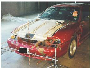
Figure 5: Case vehicle's frontal damage viewed from left of center showing underride damage pattern; Note: contour gauge at bumper level (case photo #07)
