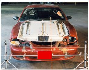
Figure 4: Elevated view of case vehicle's front underride damage with contour gauge at bumper level; Note: exposed inner hood structure and damaged headlight and turn signal assemblies (case photo #05)
