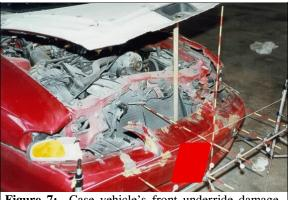
Figure 7: Case vehicle's front underride damage viewed from right of center; Note: scraping damage on top of bumper and crush to radiator (case photo #15)
