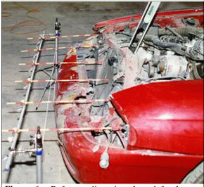
Figure 6: Reference line view from left of case vehicle's front underride damage; Note: contour gauge shows above bumper damage (case photo #09)
