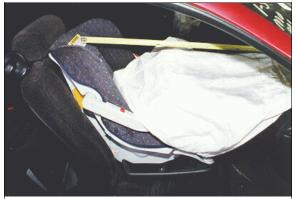
**Figure 11:** Case vehicle's outstretched, untethered, front right passenger air bag; Note: air bag's rearward excursion is capable of touching the seat back of this convertible, forward facing configured, child safety seat (case photo #34)
