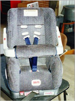
Figure 14: Front of case vehicle's undamaged Evenflo "Ultara I" convertible child safety seat; Note: harness straps improperly located when seat used in forward facing mode (case photo #40)
