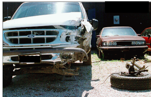
Figure 5: Other vehicle's front left damage; Note: left front wheel torn off during impact with case vehicle (case photo #30)
