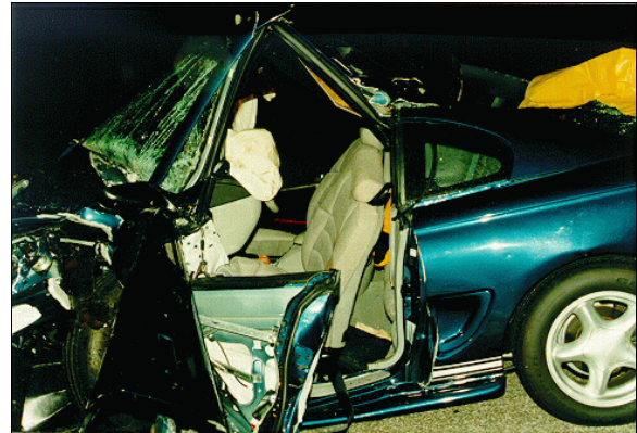
Figure 3: Intruding components of case vehicle into driver space; Note: left front tire post-crash location at lower A-pillar (case photo #12)
