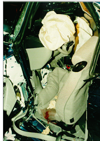
Figure 5: Case vehicle's intruded driver seating area; Note: leading edge of seat (case photo #17)
