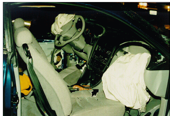
Figure 4: Interior view of case vehicle; Note: damage to steering column and wheel rim (case photo #18)
