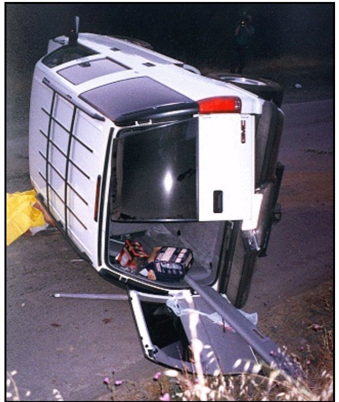
Figure 4. Exterior, case vehicle. Show rollover contact to entire left side.
