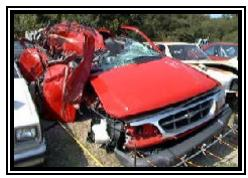
Figure 3. Front right damage (narrow end engagement) to the 1999 Ford Explorer XLT.
