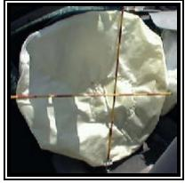
Figure 6. 1999 Ford Explorer XLT deployed redesigned driver air bag.
