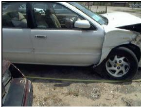
**Figure 6:** Case vehicle's right front side damage from guardrail contact (case photo #ID=70040)
