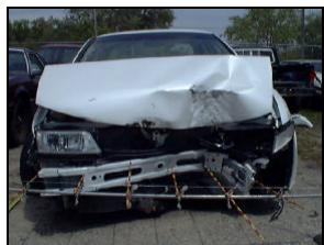
**Figure 9:** Case vehicle's front damage; Note: front left damage is from impact #5, while the front center damage is from impact #6
