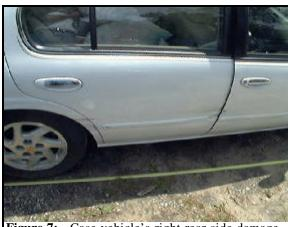
**Figure 7:** Case vehicle's right rear side damage from guardrail contact (case photo #ID=70039)
