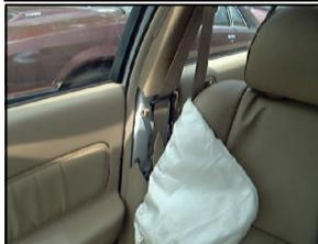
Figure 11: Case vehicle's lower right B-pillar damage from module cover flap contact
