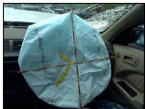
Figure 12: Case vehicle's front right passenger front air bag; Note: yellow tape outlines presence of blood and mucus on the fabric
