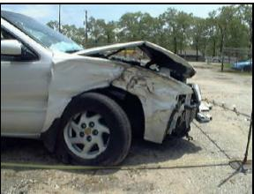
**Figure 8:** Case vehicle's right front fender damage from impact #4's sideswipe with a tree
