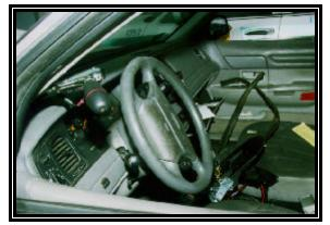
Figure 4: View of the non-deployed SRS and compressed steering column.
