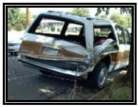
Figure 5. Right rear view of the Caravan's damage.
