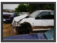
Figure 4. Profile view of the damage pattern to the Ford Explorer.
