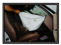
Figure 10. Excursion of the passenger air bag and adjusted position of the seat.
