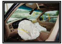
Figure 7. Deployed frontal air bag system.
