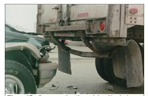
Figure 17: On-scene view from right of back showing Great Dane trailer's deformed underride guard and underride damage to case vehicle's front (case photo #51)
