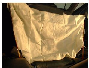
**Figure 11:** Front surface of case vehicle's deployed front right passenger air bag showing no obvious evidence of damage or contact (case photo #29)
