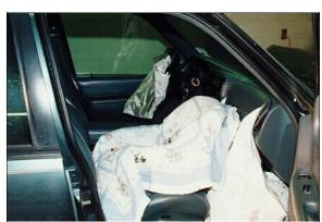
**Figure 14:** Case vehicle's front seating area showing deployed air bags and child safety seat's location in front right seat (case photo #37)
