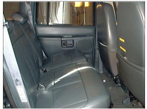
**Figure 7:** Case vehicle's back seating area showing scuff to front right seat back from unrestrained back right passenger (case photo #28b)
