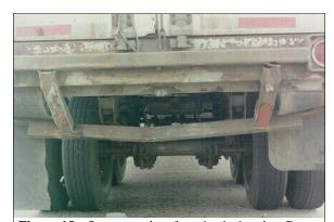
**Figure 18:** On-scene view from back showing Great Dane's deformed underride guard; Note: broken welds on underride guard (case photo #53)
