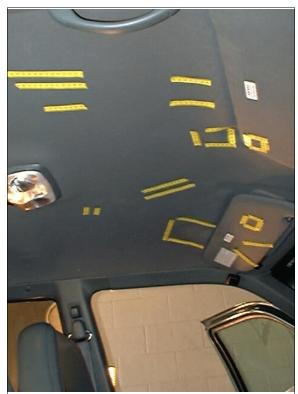
Figure 5: Vertical view from right of contact evidence on case vehicle's sun visors and roof (case photo #23)
