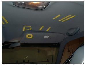
**Figure 16:** Case vehicle's right sun visor and roof contacts from child safety seat and seat's infant (case photo #26)
