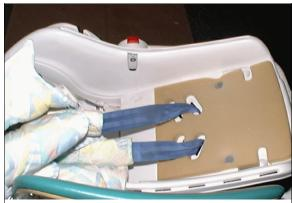
**Figure 13:** Overhead view of interior shell of case vehicle's infant child safety seat showing no evidence of damage to seat during crash; Note: seat cover removed (case photo #44)
