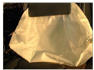
**Figure 10:** Top surface of case vehicle's deployed front right passenger air bag showing no obvious evidence of damage or contact (case photo #30)
