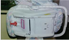
**Figure 12:** Backside of case vehicle's infant child safety seat showing no evidence of damage to seat during crash sequence (case photo #42)
