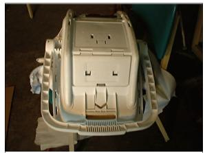
Figure 15: Undamaged back and carrying handle of case vehicle's rear facing child safety seat which was toward front right air bag module's cover flap (case photo #43)
