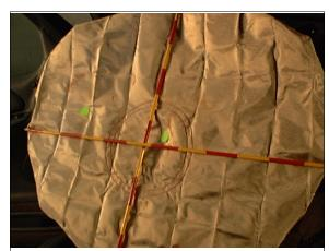
**Figure 9:** Case vehicle's deployed driver air bag showing areas containing makeup smears (i.e., dots) and blood transfers (case photo #21)
