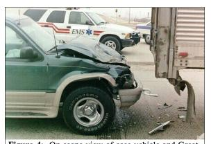
Figure 4: On-scene view of case vehicle and Great Dane's trailer at final rest; Note: trailer's underride guard damaged and bent underneath trailer (case photo #04)
