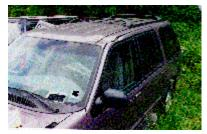
Figure 7. Secondary damage to the left roof area.
