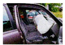
Figure 4. Profile view of the front passenger's seated position and the deployed air bag.
