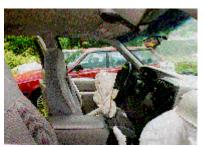
Figure 11. Right profile view of the driver's seat position and the deployed air bag.
