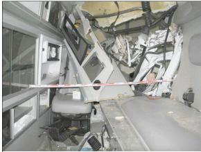
Figure 7: Intruding components into the patient compartment
