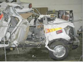
**Figure 3:** Initial contact with the tree began on the right fender of the ambulance
