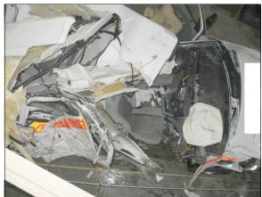
**Figure 5:** Top view of the crush sustained by the ambulance and the displacement of the right Apillar and door frame
