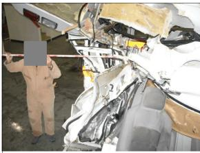
**Figure 6:** Front to rear view of the crush at the ambulance's right roof side rail
