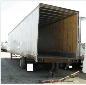
**Figure 1:** The damaged 2008 Wabash National semitrailer and its damaged rear impact guard
