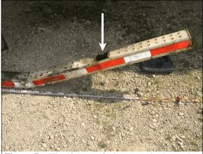
**Figure 7:** The right vertical support broke at the weld on the impact guard
