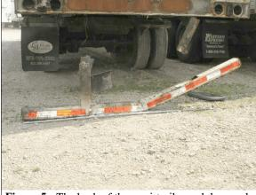
Figure 5: The back of the semi-trailer and damaged impact guard
