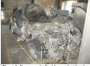
**Figure 4:** Damage on the Ford from underriding the semi-trailer and from the fire
