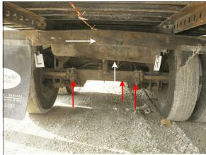
**Figure 6:** The Ford contacted the mud flap bracket, air reservoir tank, slack adjusters, and the axle
