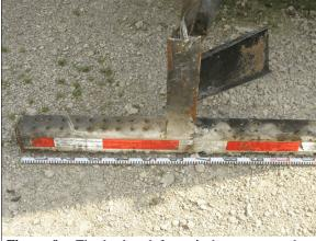
Figure 9: The broken left vertical support on the impact guard
