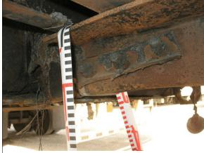
**Figure 10:** The broken impact guard vertical support bracket on the left frame rail of the semi-trailer
