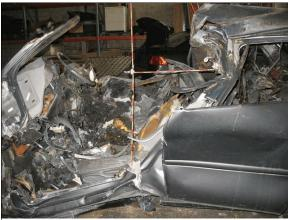
Figure 11: Left side view of the roof and A-pillar crush on the Ford
