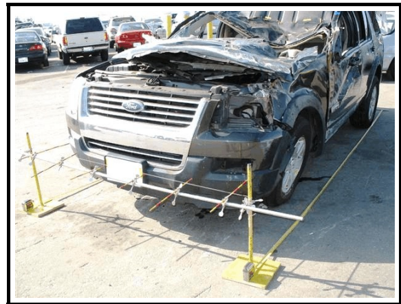
Figure 3. Front end crush profile measurement
