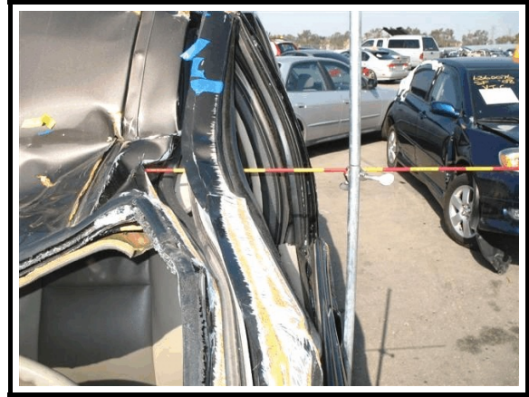
Figure 4. Maximum lateral crush measurement, left roof side rail
