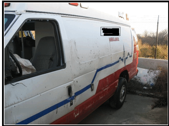
Figure 6. Left side rollover damage
