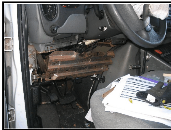
Figure 12. Deformed knee bolster
