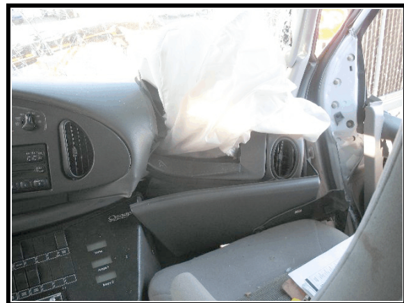
Figure 7. Right interior intrusion
