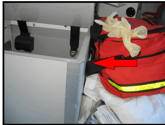
Figure 17. Deformation to upper right corner of seat support
