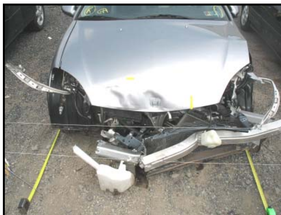
Figure 4: View of the frontal damage.
