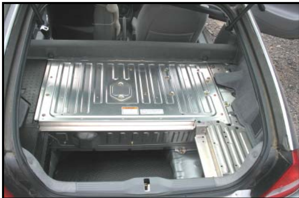
Figure 10: Battery compartment and storage well.
