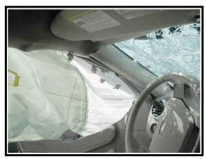
**Figure 9**. Contact to interior portion of curtain
