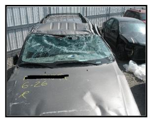
Figure 6. Rollover damage to top
