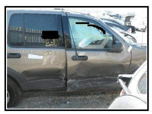
Figure 4. Right side damage
