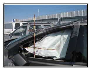
Figure 8. Damage to curtain exterior
