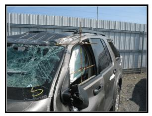
Figure 5. Maximum vertical crush
