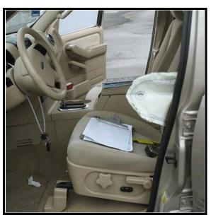
**Figure 9**. Seat-mounted side air bag, outboard view
