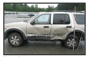
**Figure 5**. Left side damage from impact with Saab
