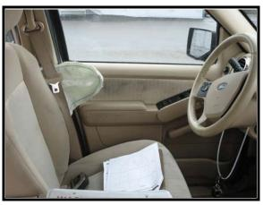
Figure 8. Side air bag, inboard view
