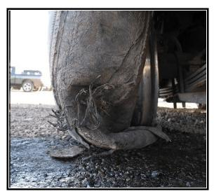
Figure 6. Left rear tire, from back
