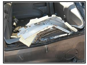
**Figure 9**. Fracture and displacement of interior left side panel
