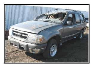
**Figure 7**. View showing crush to roof
