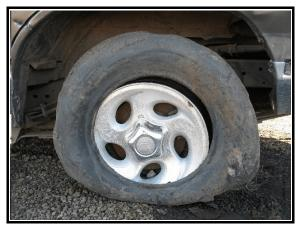
**Figure 2**. Left rear tire sustained tread separation
