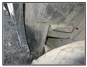
**Figure 8**. Rubber transfer to inner wheel well
