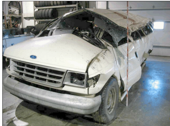
Figure 6: Overview of damage to Ford's top and left side; vertical scale in tenths of meter
