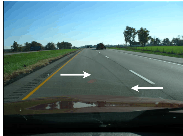
Figure 1: Approach of Ford southbound in inside lane; right arrow shows Ford’s right rear yaw mark, left arrow shows right front yaw mark
