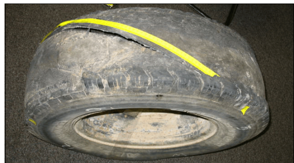
Figure 15: Tear in carcass of Ford's left rear tire
