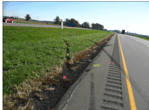
Figure 2: Ford’s yaw marks departing inside shoulder of southbound lanes into median, yaw marks from right to left are right rear, left rear and right front
