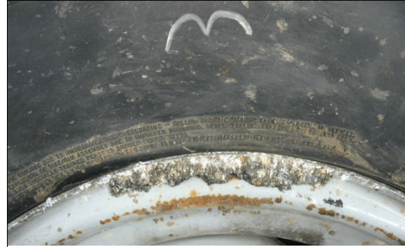
Figure 17: Dent in rim flange on outboard side of Ford's left rear wheel with bituminous jammed in flange; dent formed by force directed parallel to axle
