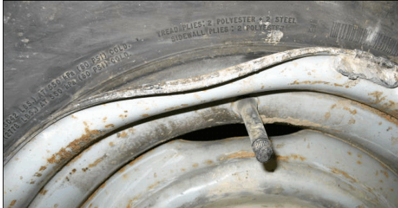
Figure 16: Dent in rim flange on outboard side of Ford's left rear wheel, dent formed by force directed toward center of rotation
