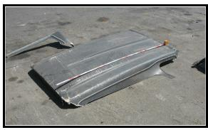
**Figure 10**. Contact damage to top of box cap
