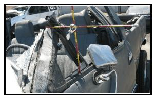
Figure 8. Crush at left A pillar area
