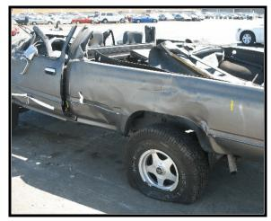
**Figure 11**. Left side contact damage from Event 1
