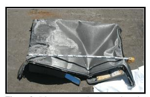
**Figure 9**. Direct contact damage and crush to cab roof
